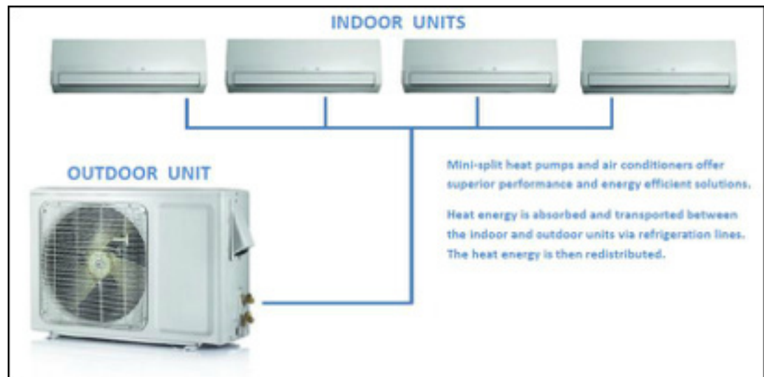
Schematic of Multi-Zone Mini-Split System
