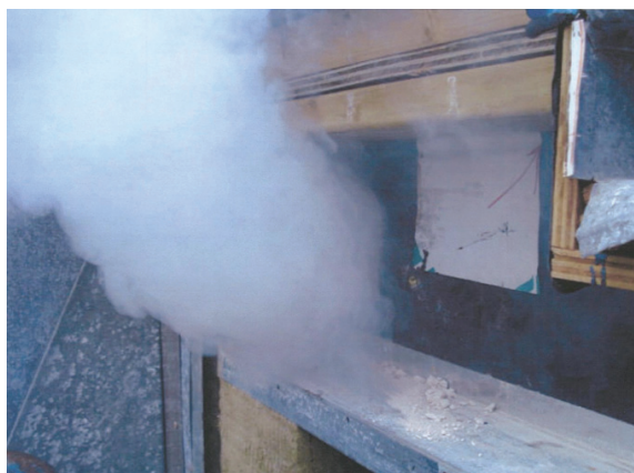
Qualitative (smoke tracer) airtightness testing of a parapet detail mock-up
