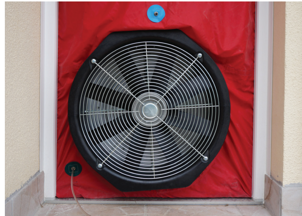
High-powered blower fan installed in a door opening
