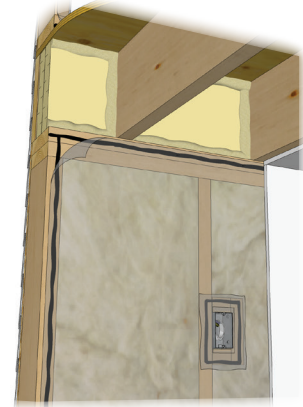
Sealed polyethylene approach
