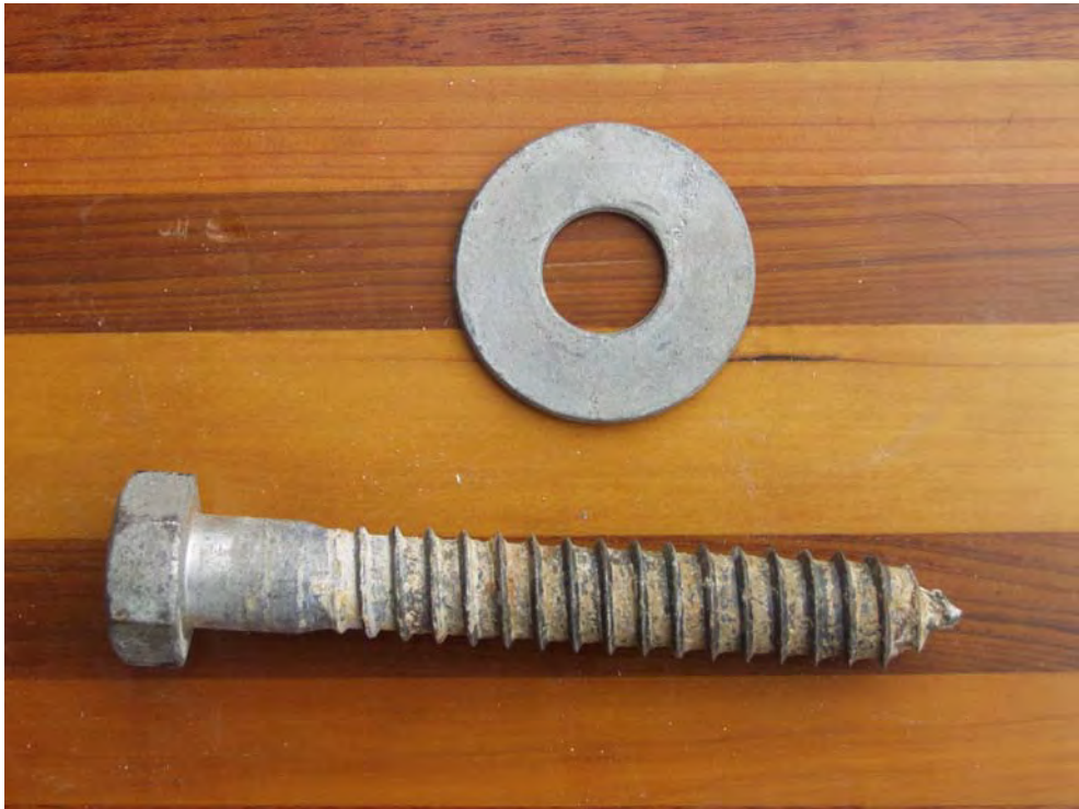
Figure 63. Galvanized lag bolt removed from deck bracket into ACQ rim joist.
