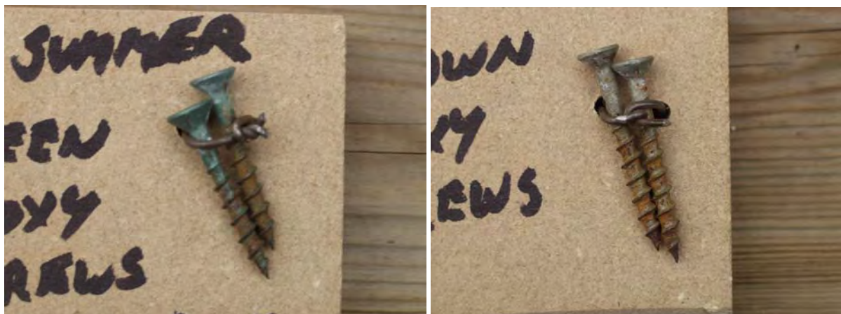
Figure 57. Corrosion of green and brown epoxy coated decking screws
