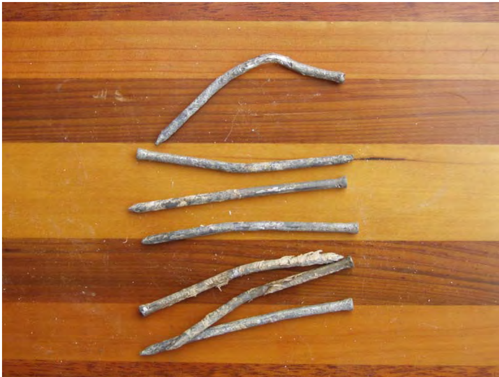
Figure 62. Galvanized casing nails removed from ACQ stair tread
