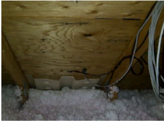
Photo 12: Sensor Set-up At Baffles
