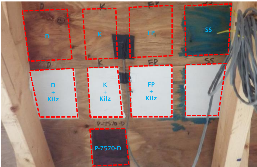
Figure 2.3 Example surface biocide treatment on the underside of the roof sheathing
