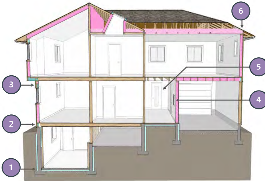
Figure 2: Typical Problem Areas for Insulation Continuity
