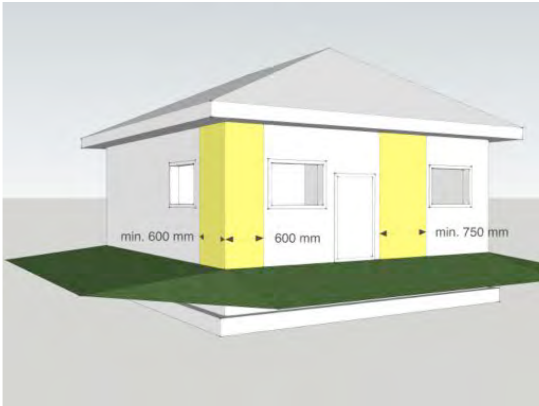
Minimum length of braced wall panels when connecting to intersecting braced wall panels, and minimum panel length in the field of the wall. x
