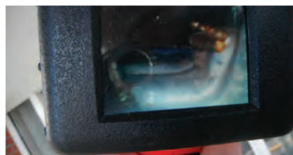
Scoped cameras provide views of duct interiors.
