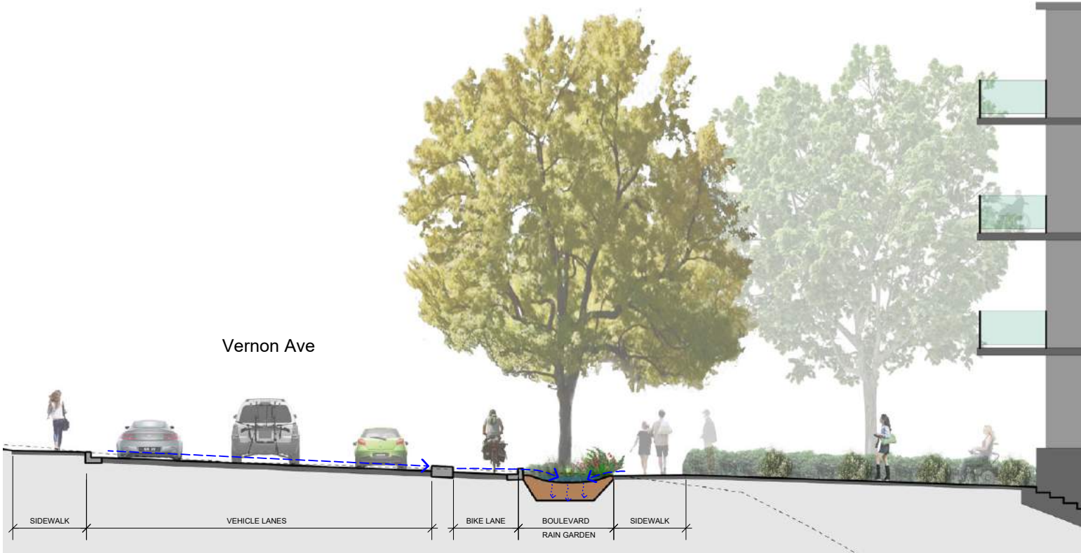
Typical Section: Reduce to 3 Travel Lanes
