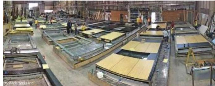
Figure 31 - Full scale mock-up testing of the building envelope panels (©Azadeh Fallahi)
