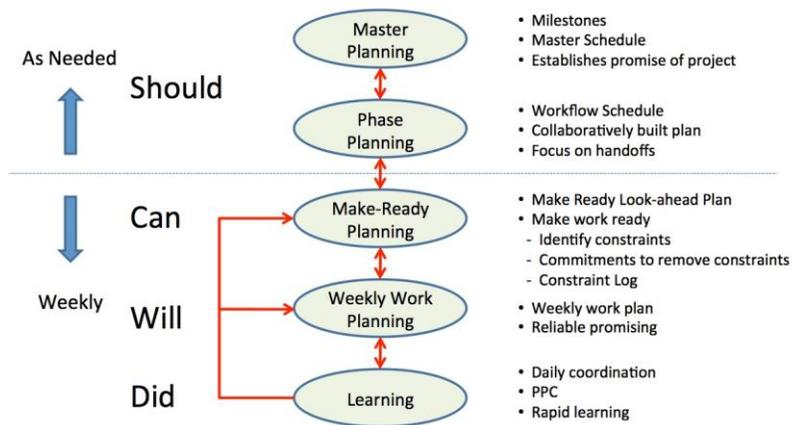
Figure 8 - Last Planner System (source Lean Construction Blog)
