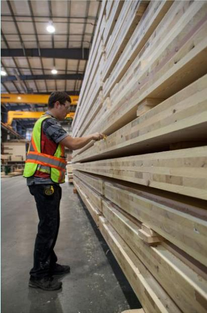
Structurlam, the mass-timber supplier for Brock Commons, is an industry leader in the application of comprehensive 3D modelling with digital fabrication of innovative structural solutions. Leveraging their established BIM capabilities, they were able to take advantage of available models for digital fabrication of the mass timber elements (Image source Wood Innovates BC<sup>55</sup>).
