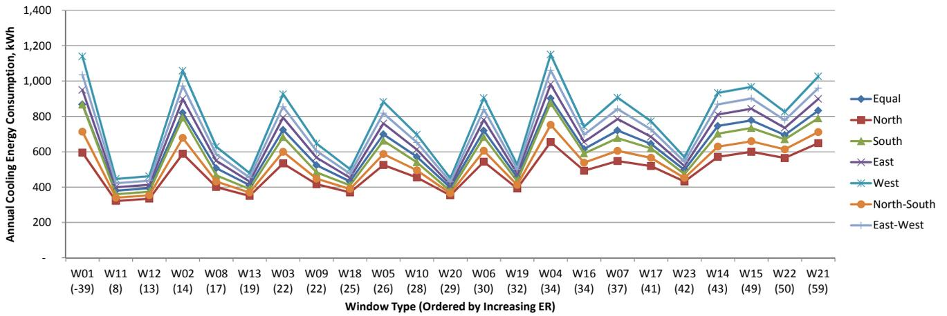
Fig.7.60 Annual cooling energy consumption for window orientations in Vancouver, kWh.
