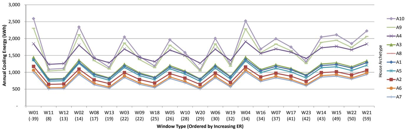
Fig.7.36 Annual cooling energy consumption for archetype houses in Montreal, kWh.
