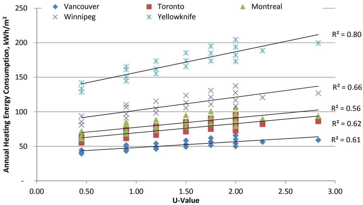
Fig.11.36 Annual heating energy versus U-Value, 60% WWR, kWh/m<sup>2</sup>.
