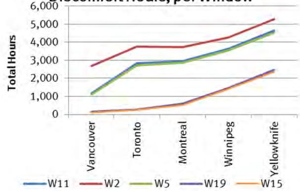
Fig. 9.5.35 E1, Average window surface temperature discomfort hours compared with D1
