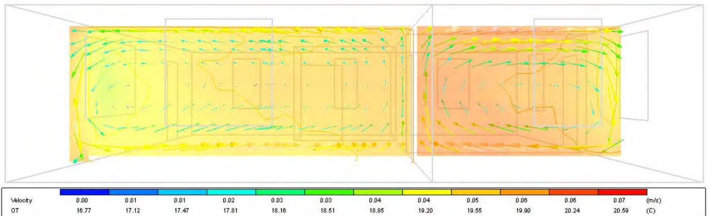
Fig. 9.6.5 CFD Results: Operative temperature distribution in Vancouver, W2 and W15
