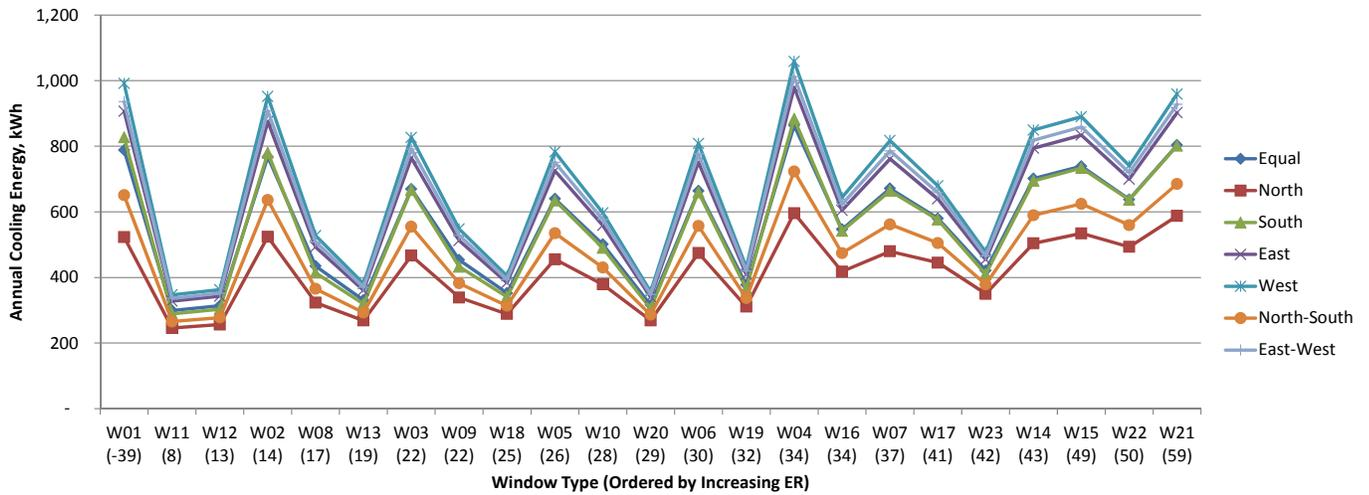
Fig.7.72 Annual cooling energy consumption for window orientations in Yellowknife, kWh.
