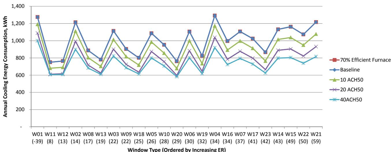
Fig.7.92 Annual cooling energy consumption in Toronto, kWh.
