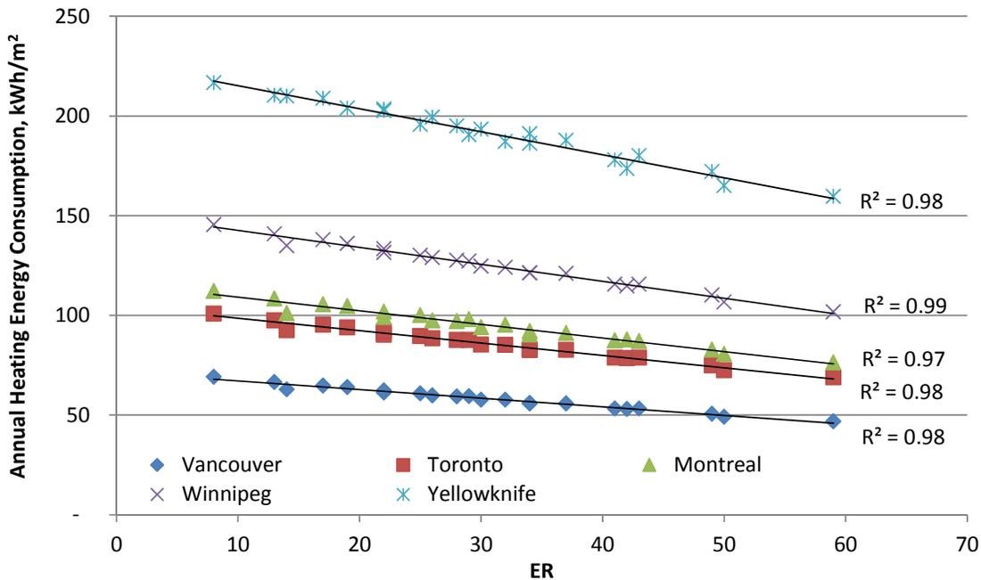
Fig.11.21 Annual heating energy consumption versus ER, 40% WWR, kWh/m<sup>2</sup>.
