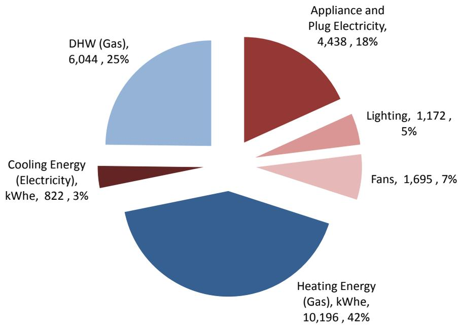
Fig.11.1 Distribution of row house end unit (north-south) household energy consumption in Vancouver, kWh<sub>e</sub> and percent of total.
