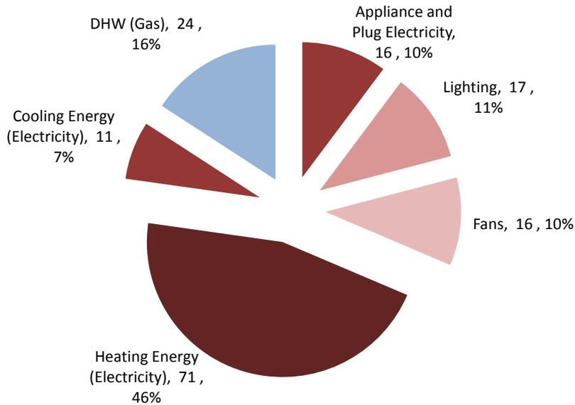
Fig.11.25 Distribution of high-rise building energy consumption in Vancouver, 40% WWR, kWh<sub>e</sub>/m<sup>2</sup> and percent of total.
