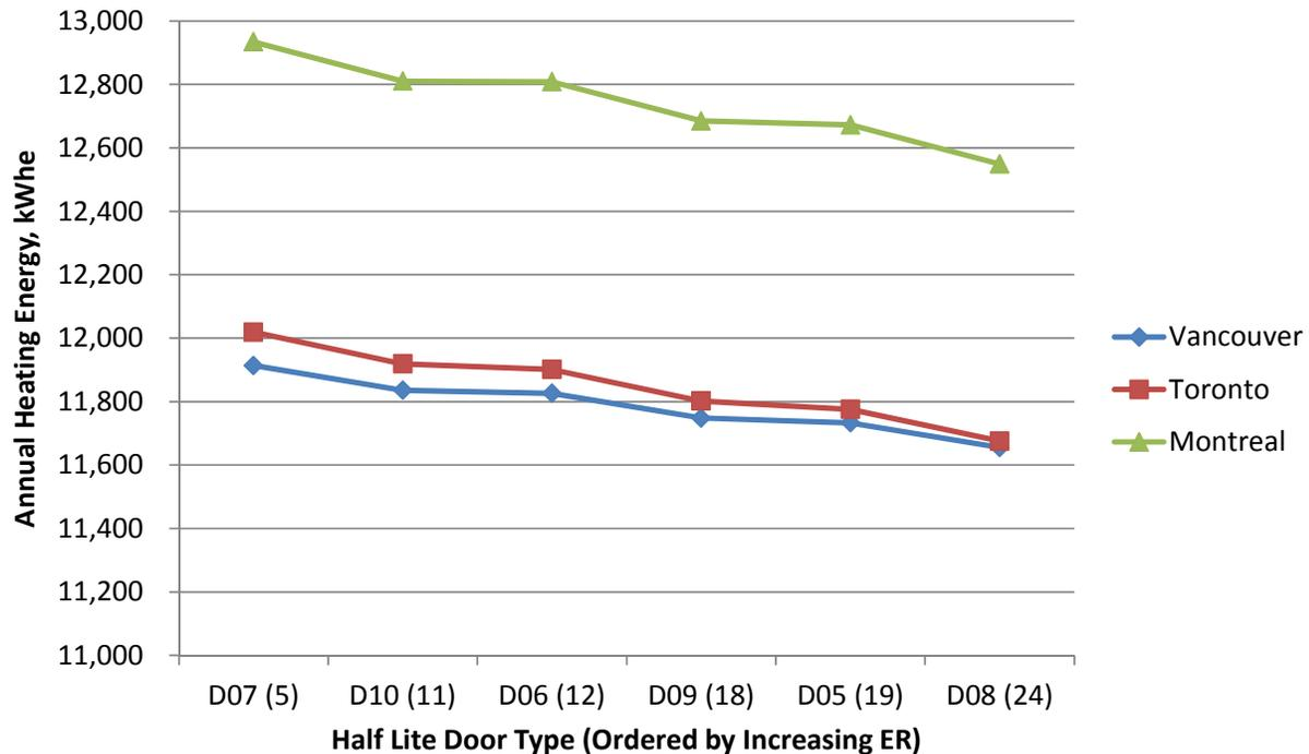
Fig.10.13 Annual heating energy consumption of half lite doors, Vancouver, Toronto and Montreal, kWh<sub>e</sub>.
