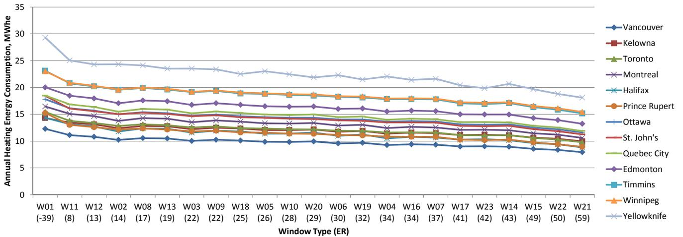
Fig.7.24 Annual heating energy consumption, MWh<sub>e</sub>.
