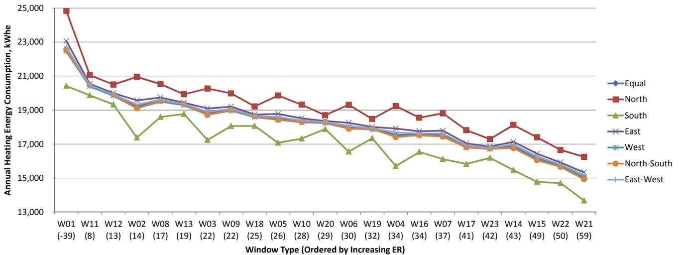
Fig.7.68 Annual heating energy consumption for window orientations in Winnipeg, kWh<sub>e</sub>.
