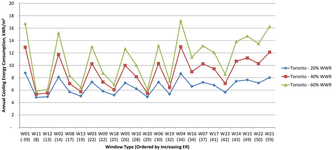
Fig.11.19 Annual cooling energy consumption for low-rise building in Toronto, kWh/m<sup>2</sup>.
