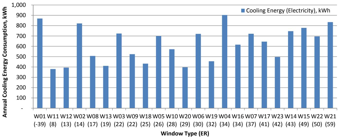
Fig.7.16 Annual cooling energy consumption in Vancouver, kWh.
