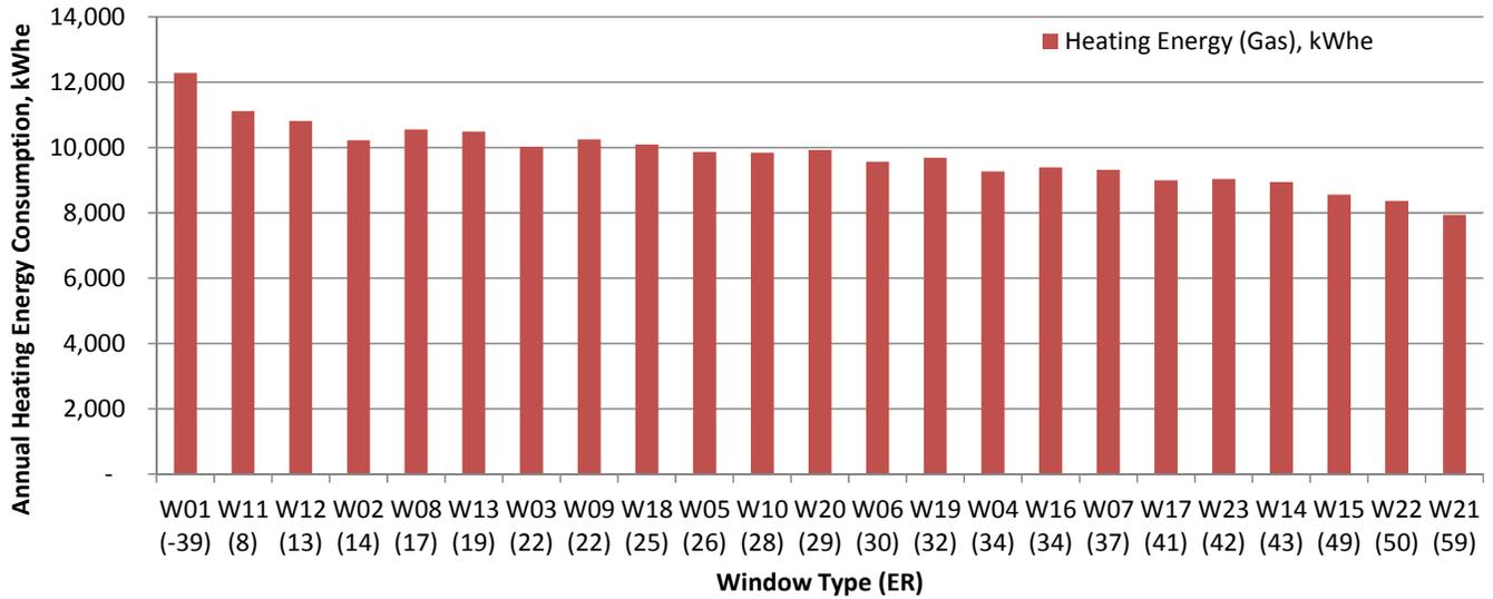
Fig.7.15 Annual heating energy consumption in Vancouver, kWh<sub>e</sub>.
