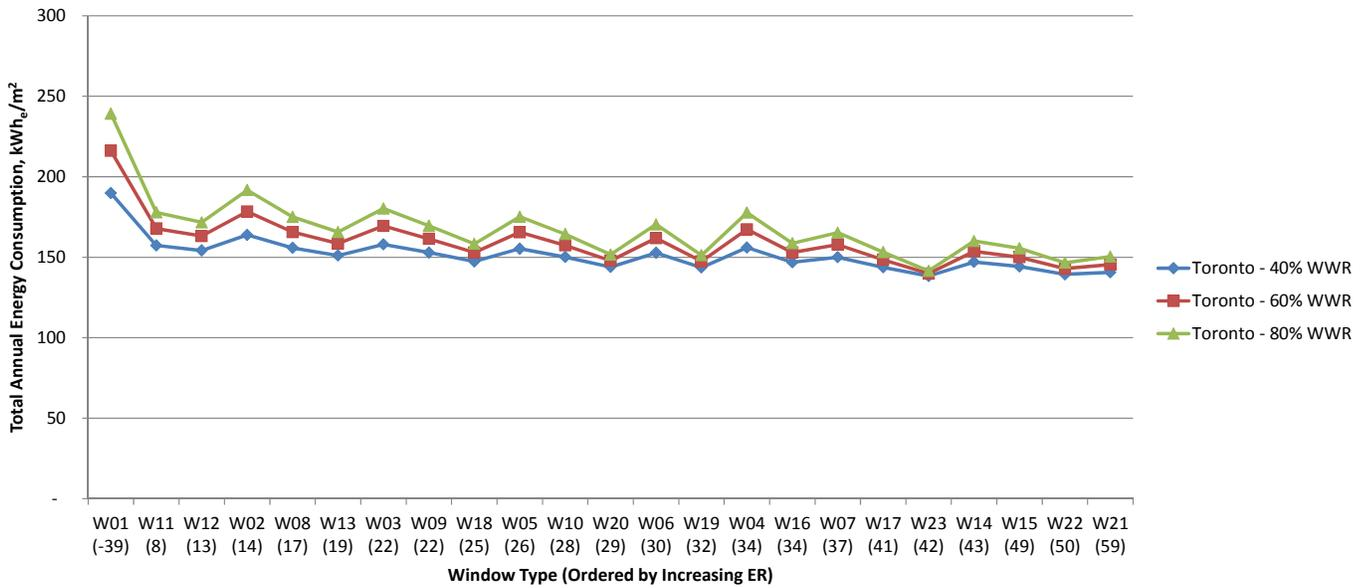
Fig.11.33 Total annual energy consumption for high-rise building in Toronto, kWh<sub>e</sub>/m<sup>2</sup>.
