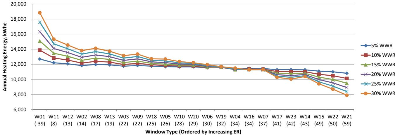
Fig.7.47 Annual heating energy consumption for window to wall ratios in Toronto, kWh<sub>e</sub>.
