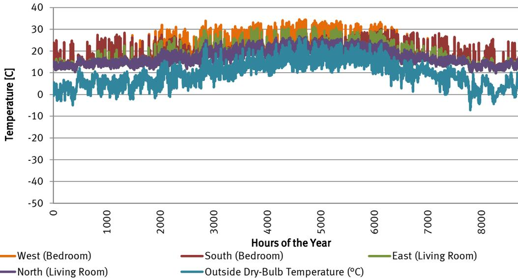
Fig. 9.4.5 D1 Vancouver, Window surface temperatures
