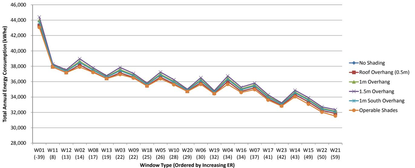
Fig.7.90 Total annual energy consumption for window shading scenarios in Yellowknife, kWh<sub>e</sub>.
