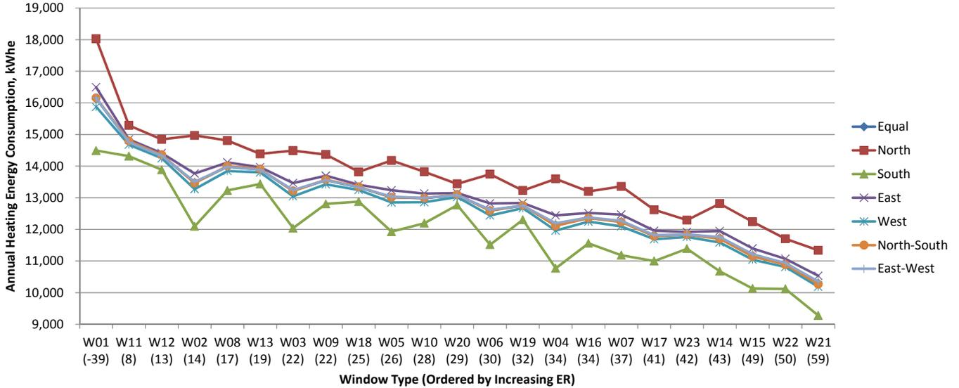
Fig.7.65 Annual heating energy consumption for window orientations in Montreal, kWh<sub>e</sub>.
