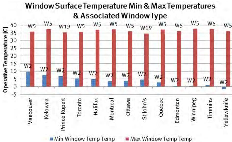
Fig. 9.6.3 Minimum & maximum window surface temperatures per city
