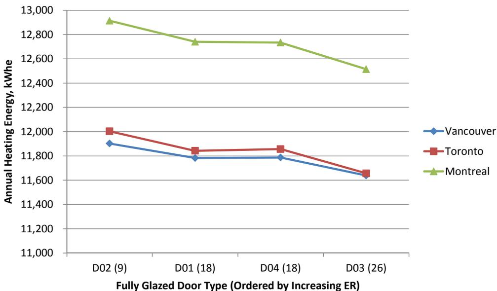
Fig.10.9 Annual heating energy consumption of fully glazed doors, Vancouver, Toronto and Montreal, kWh<sub>e</sub>.
