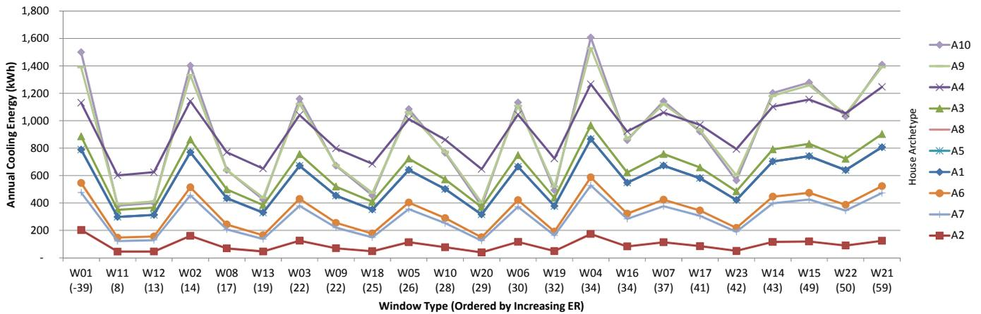
Fig.7.42 Annual cooling energy consumption for archetype houses in Yellowknife, kWh.
