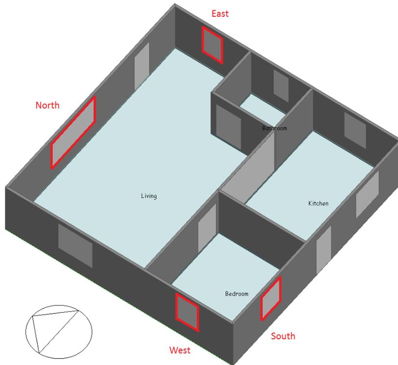
Fig. 9.3.2 Windows used for Surface Temperature Analysis
