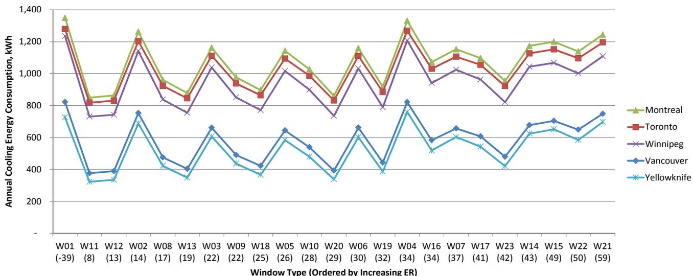
Fig.11.5 Annual cooling energy consumption, end unit archetype facing north-south, kWh.
