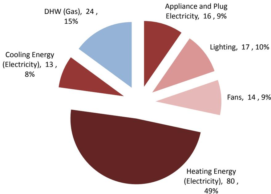
Fig.11.27 Distribution of high-rise building energy consumption in Toronto, 40% WWR, kWh<sub>e</sub>/m<sup>2</sup> and percent of total.
