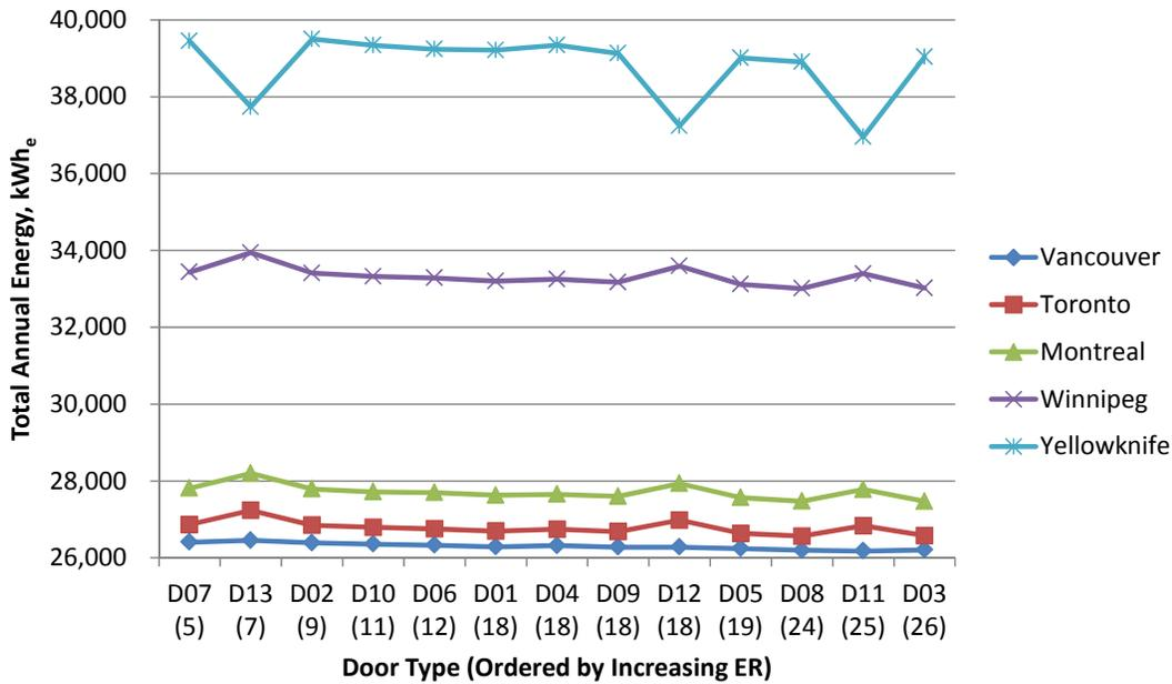
Fig.10.8 Total annual energy consumption of doors, including all door types, kWh<sub>e</sub>.
