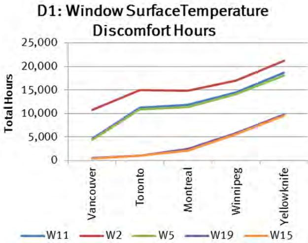
Fig. 9.5.3 D1 Total window surface temperature discomfort hours
