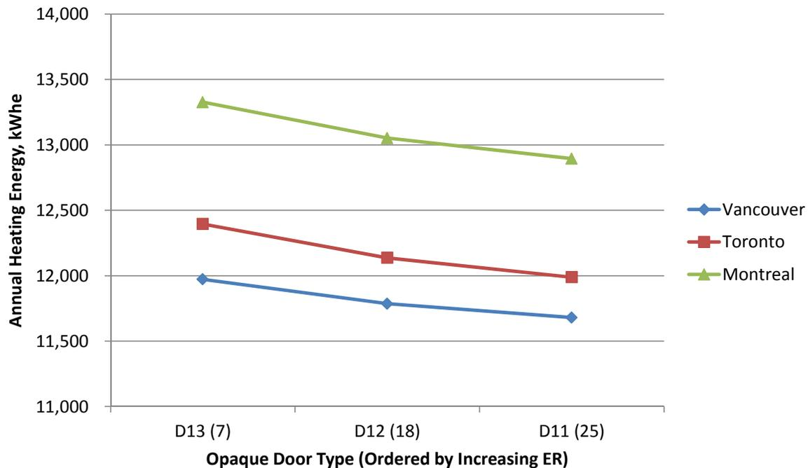
Fig.10.17 Annual heating energy consumption of half lite doors, Vancouver, Toronto and Montreal, kWh<sub>e</sub>.
