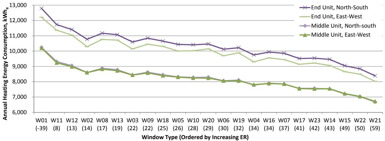
Fig.11.7 Annual heating energy consumption, row house archetypes in Toronto, kWh<sub>e</sub>.
