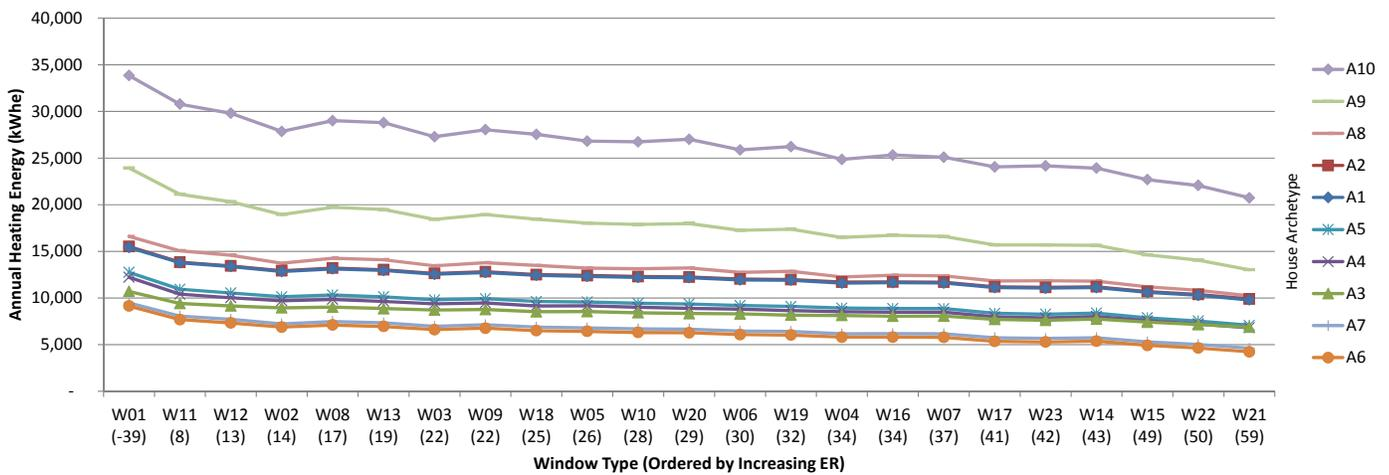
Fig.7.32 Annual heating energy consumption for archetype houses in Toronto, kWh<sub>e</sub>.
