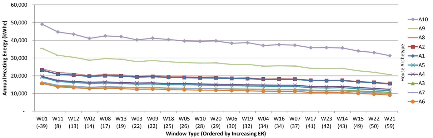
Fig.7.38 Annual heating energy consumption for archetype houses in Winnipeg, kWh<sub>e</sub>.
