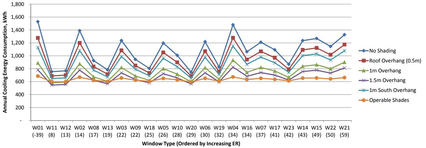
Fig.7.86 Annual cooling energy consumption for window shading scenarios in Winnipeg, kWh.
