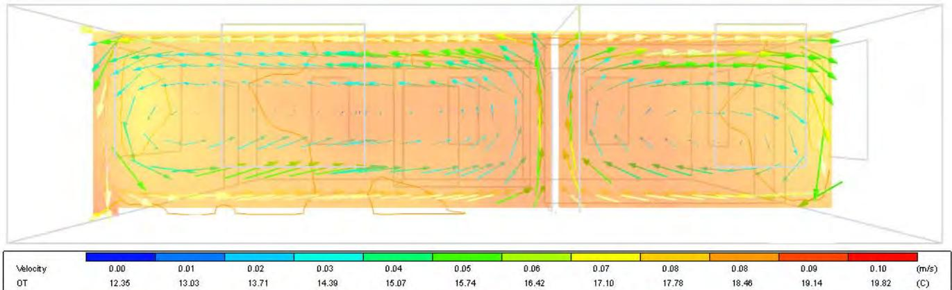
Fig. 9.6.4 CFD Results: Operative temperature distribution in Yellowknife, W2 and W15
