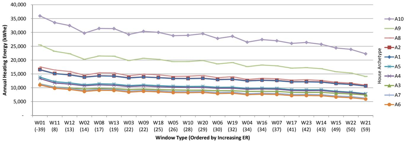
Fig.7.35 Annual heating energy consumption for archetype houses in Montreal, kWh<sub>e</sub>.
