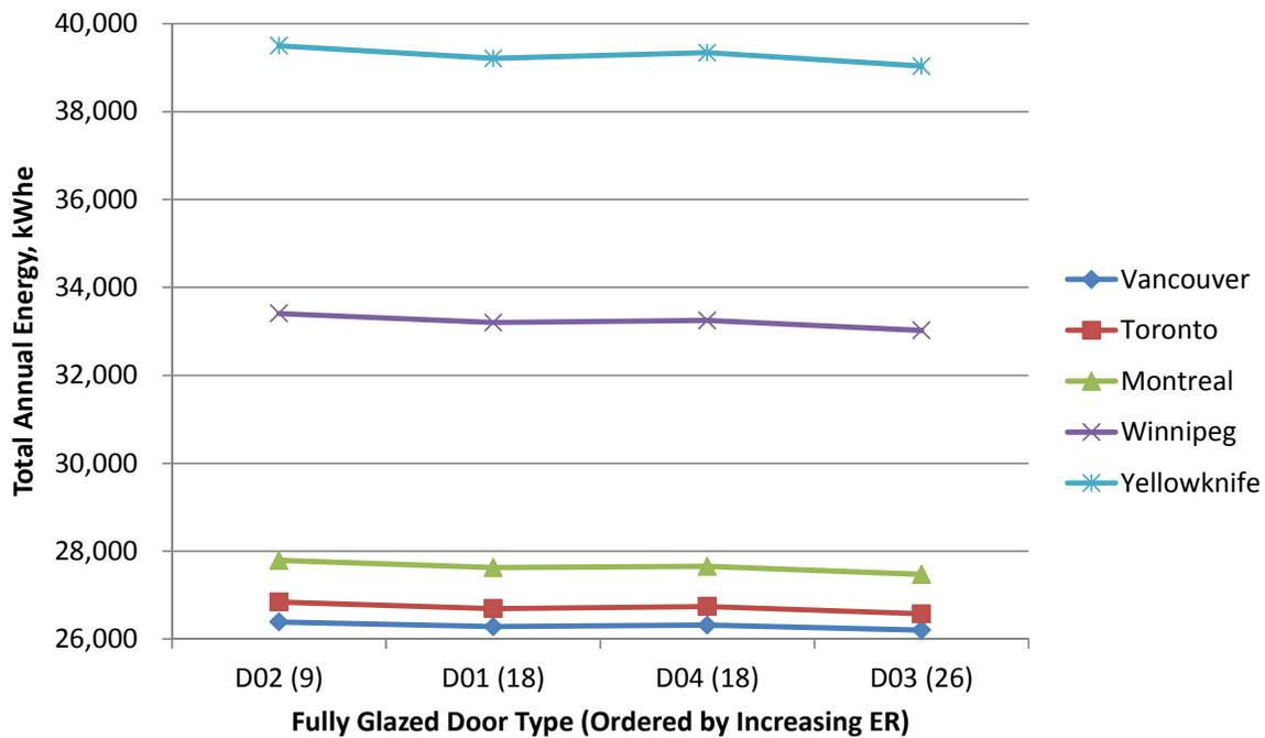
Fig.10.12 Total annual energy consumption of fully glazed doors, kWh<sub>e</sub>.
