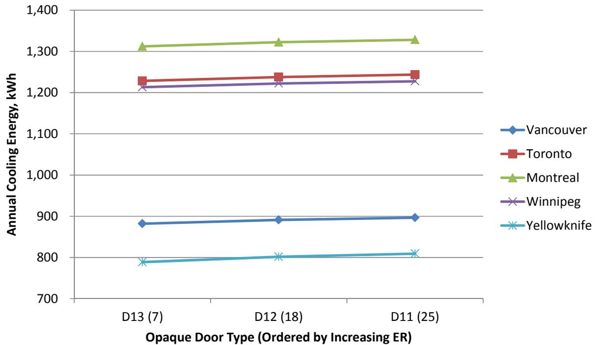
Fig.10.19 Annual cooling energy consumption of opaque doors, kWh.
