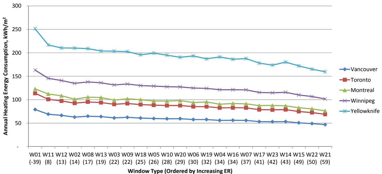
Fig.11.15 Annual heating energy consumption for low-rise building with 40% WWR, kWh/m<sup>2</sup>.
