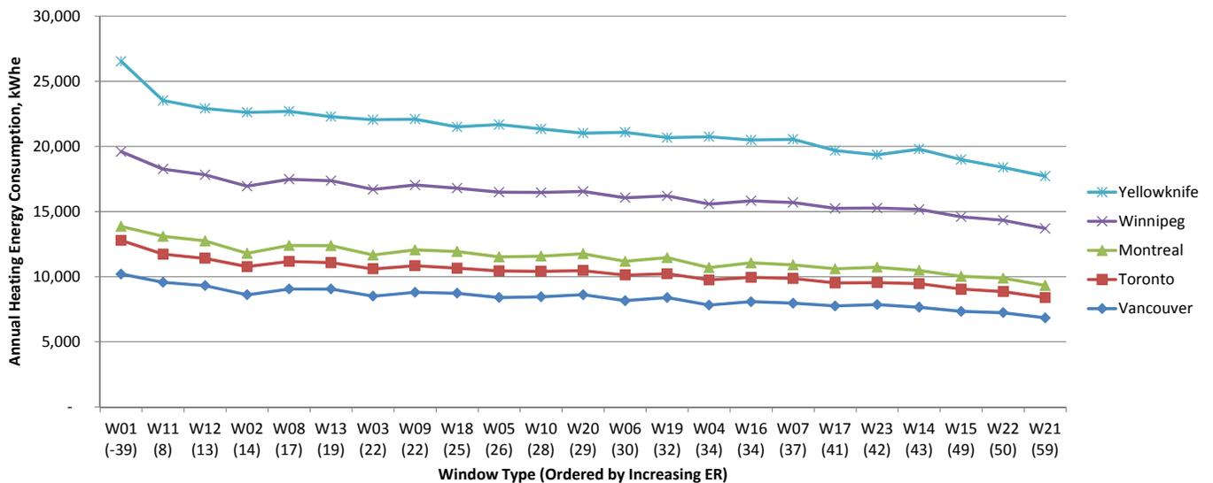
Fig.11.4 Annual heating energy consumption, end unit archetype facing north-south, kWh<sub>e</sub>.
