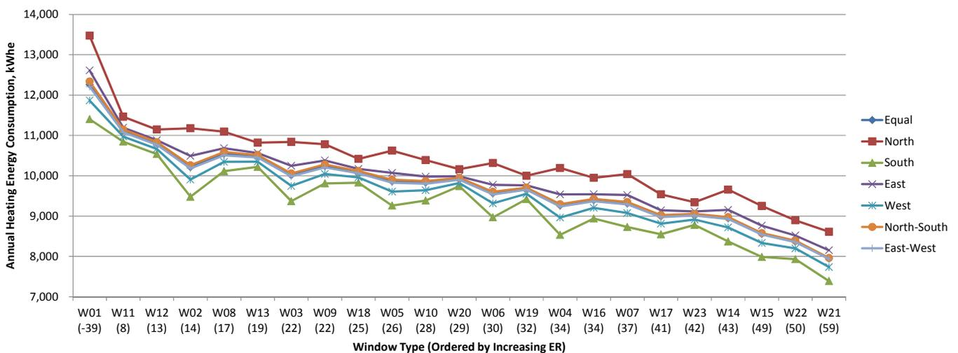
Fig.7.59 Annual heating energy consumption for window orientations in Vancouver, kWh<sub>e</sub>.
