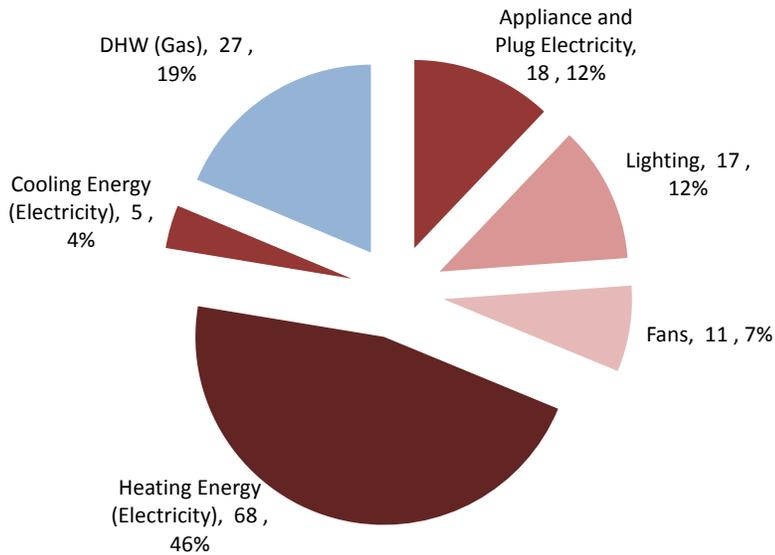
Fig.11.13 Distribution of low-rise building energy consumption in Vancouver, 20% WWR, kWh<sub>e</sub>/m<sup>2</sup> and percent of total.
