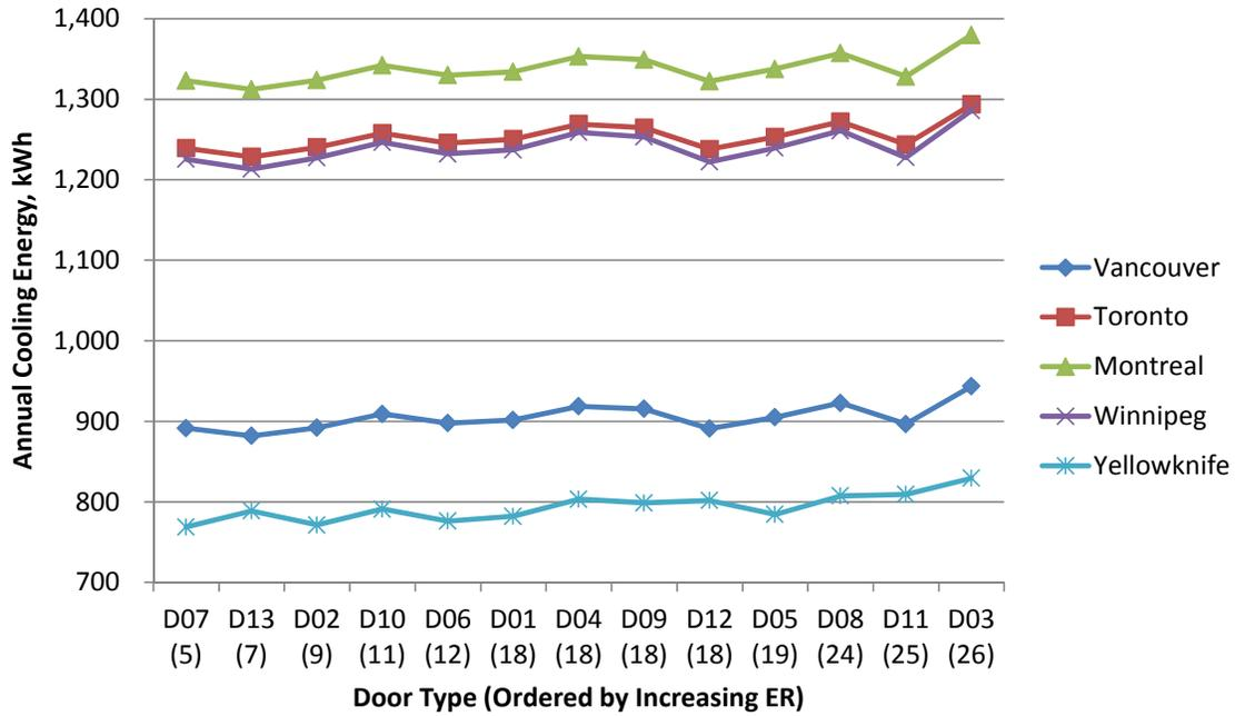
Fig.10.7 Annual cooling energy consumption of doors, including all door types, kWh.
