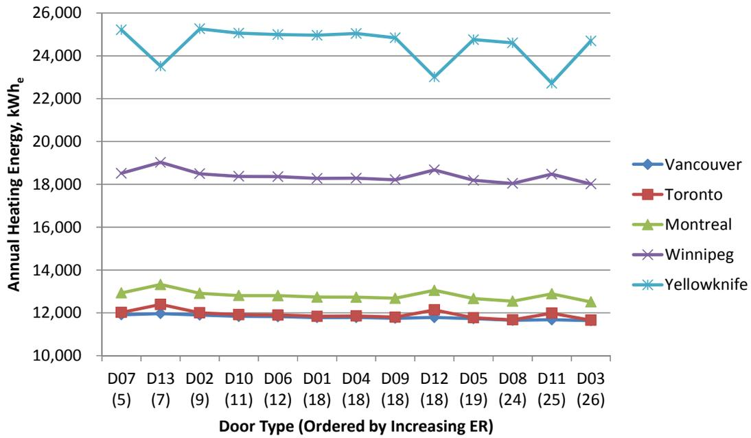
Fig.10.6 Annual heating energy consumption of doors, including all door types, kWh<sub>e</sub>.
