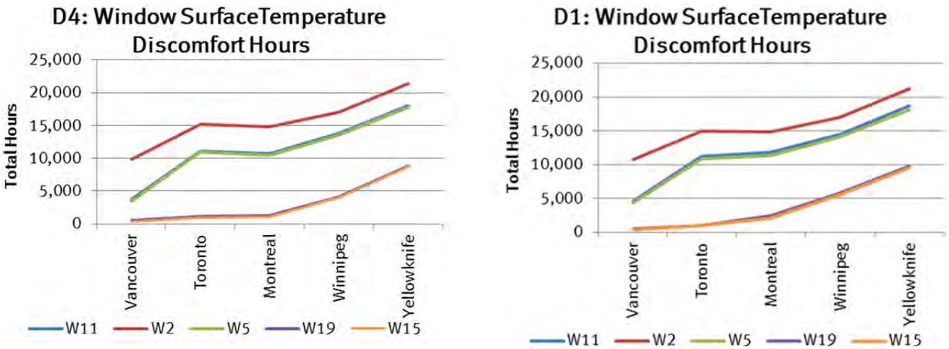
Fig. 9.5.21 D4, Window surface temperature discomfort hours compared with D1
