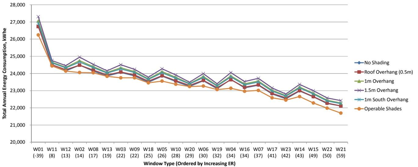
Fig.7.78 Total annual energy consumption for window shading scenarios in Vancouver, kWh<sub>e</sub>.
