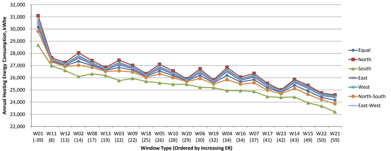
Fig.7.64 Total annual energy consumption for window orientations in Toronto, kWh<sub>e</sub>.
