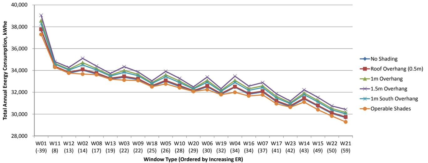
Fig.7.87 Total annual energy consumption for window shading scenarios in Winnipeg, kWh<sub>e</sub>.
