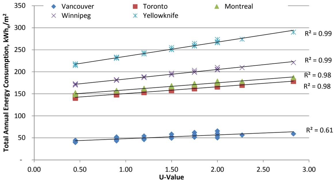
Fig.11.37 Total annual energy versus U-Value, 60% WWR, kWh<sub>e</sub>/m<sup>2</sup>.
