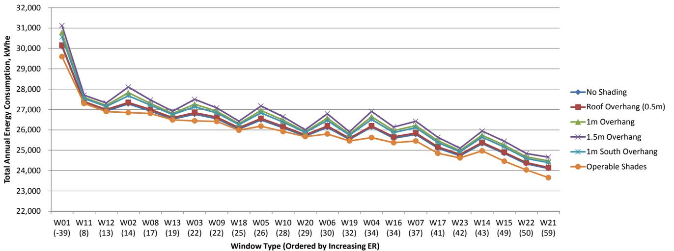
Fig.7.81 Total annual energy consumption for window shading scenarios in Toronto, kWh<sub>e</sub>.
