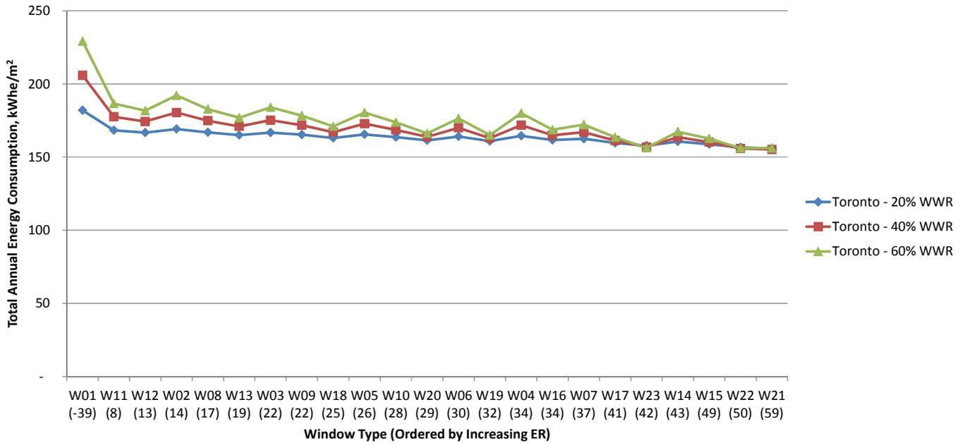
Fig.11.20 Total annual energy consumption for low-rise building in Toronto, kWh<sub>e</sub>/m<sup>2</sup>.
