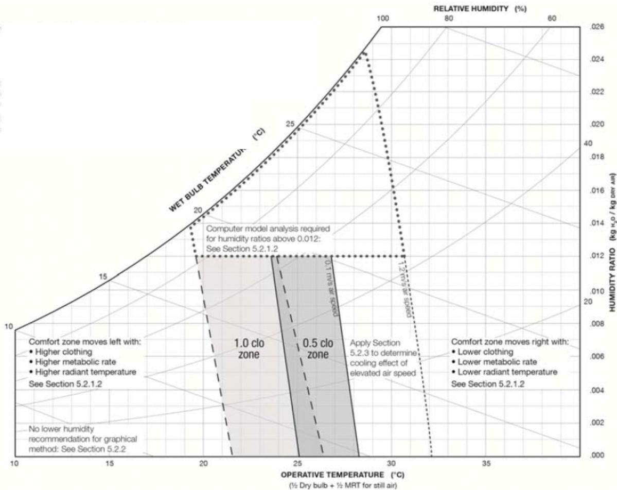
Fig. 9.3.5 ASHRAE Standard 55-2010 (Fig 5.2.1.1), thermal comfort limits.
