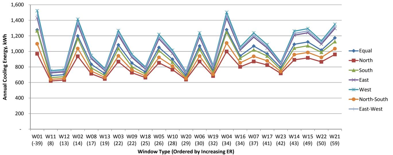
Fig.7.69 Annual cooling energy consumption for window orientations in Winnipeg, kWh.
