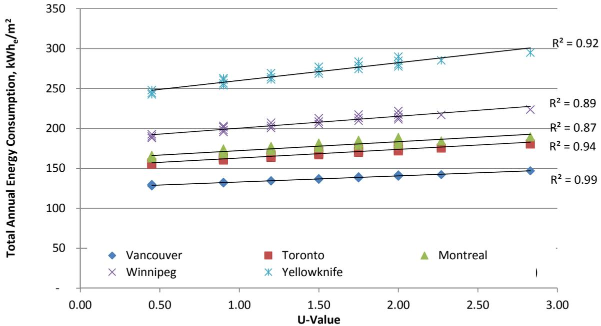
Fig.11.24 Total annual energy consumption versus U-value, 40% WWR, kWh<sub>e</sub>/m<sup>2</sup>.
