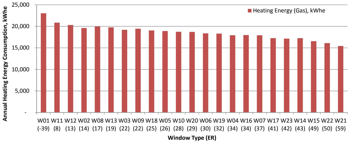
Fig.7.21 Annual heating energy consumption in Winnipeg, kWh<sub>e</sub>.
