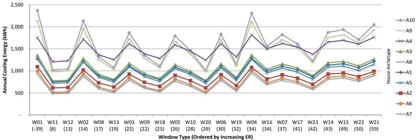
Fig.7.33 Annual cooling energy consumption for archetype houses in Toronto, kWh.
