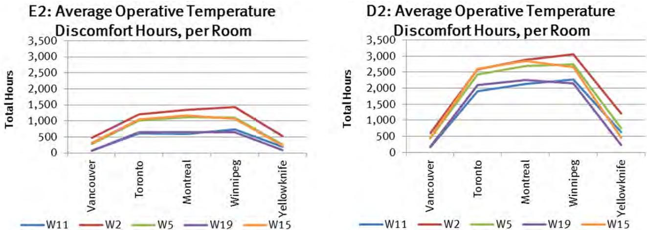
Fig. 9.5.40 E2, Operative temperature discomfort hours per room compared with D2
