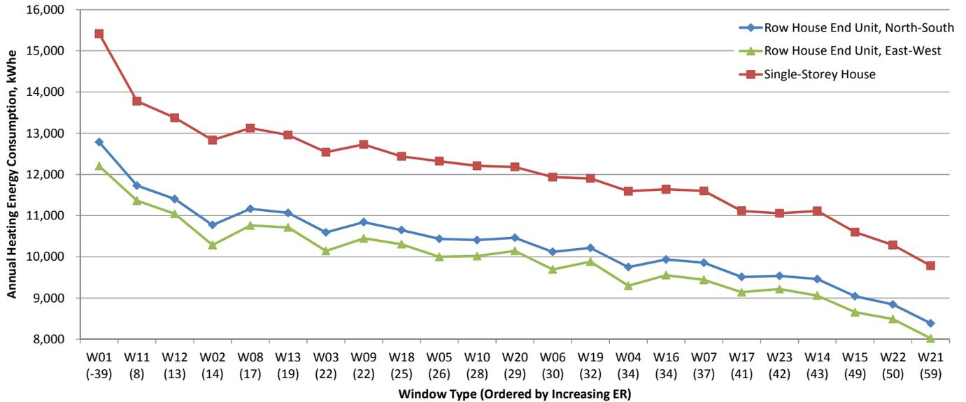
Fig.11.10 Annual heating energy consumption, row house and single-storey archetypes in Toronto, kWh<sub>e</sub>.
