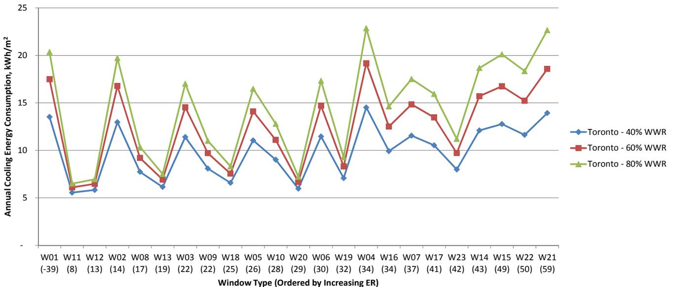
Fig.11.32 Annual cooling energy consumption for high-rise building in Toronto, kWh/m<sup>2</sup>.
