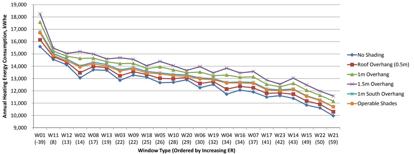
Fig.7.82 Annual heating energy consumption for window shading scenarios in Montreal, kWh<sub>e</sub>.
