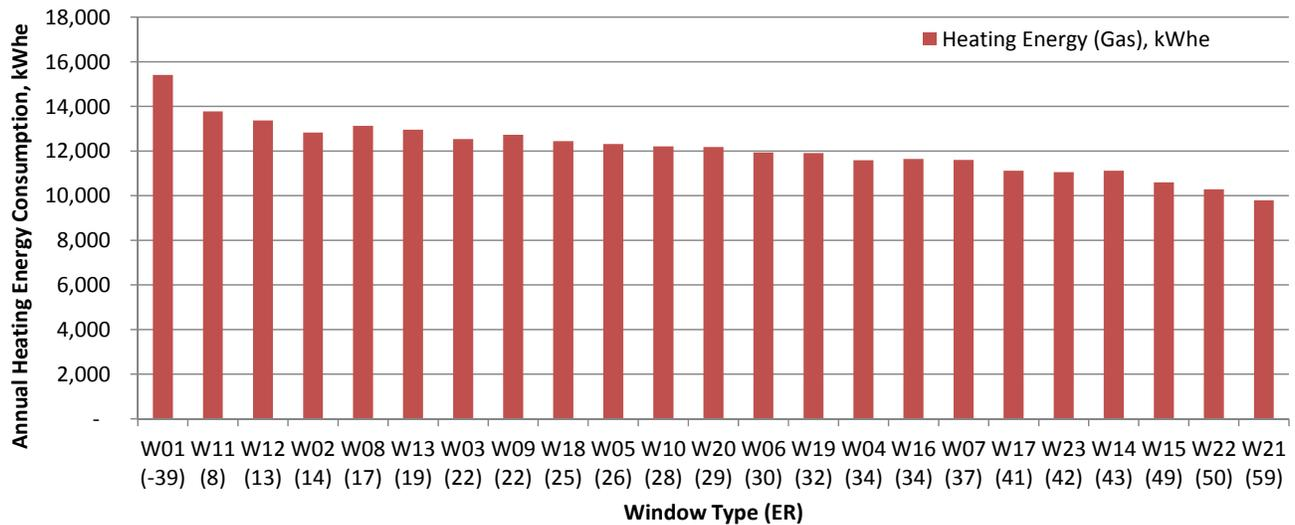
Fig.7.18 Annual heating energy consumption in Toronto, kWh<sub>e</sub>.
