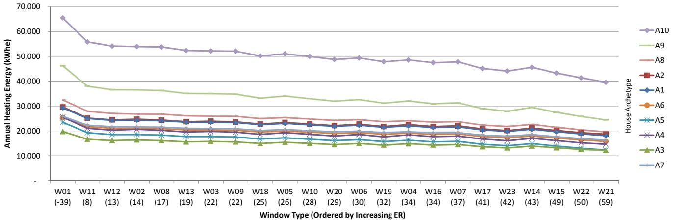
Fig.7.41 Annual heating energy consumption for archetype houses in Yellowknife, kWh<sub>e</sub>.
