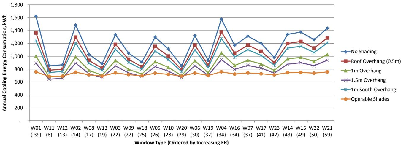
Fig.7.83 Annual cooling energy consumption for window shading scenarios in Montreal, kWh.
