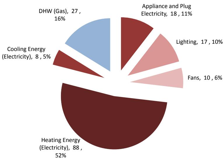
Fig.11.14 Distribution of low-rise building energy consumption in Toronto, 20% WWR, kWh<sub>e</sub>/m<sup>2</sup> and percent of total.
