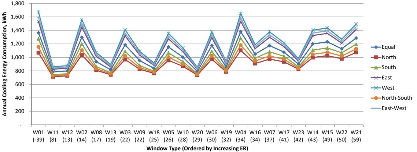
Fig.7.66 Annual cooling energy consumption for window orientations in Montreal, kWh.
