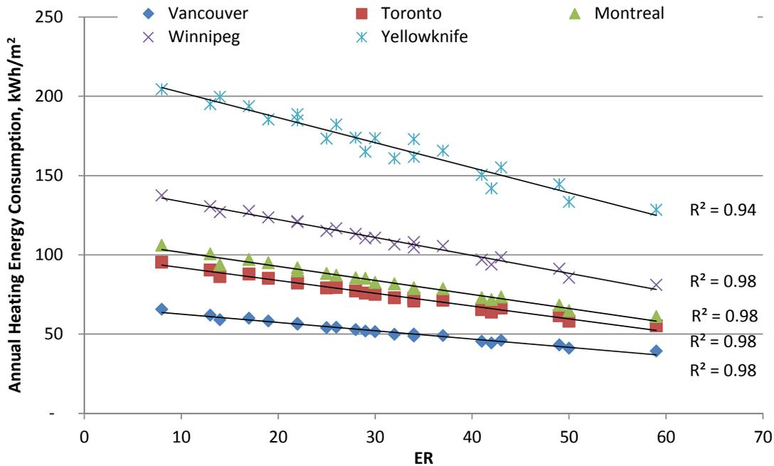
Fig.11.34 Annual heating energy versus ER, 60% WWR, kWh/m<sup>2</sup>.
