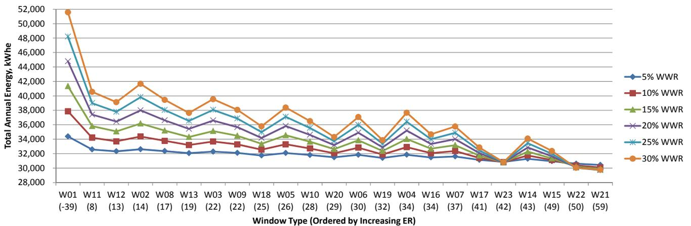
Fig.7.58 Total annual energy consumption for window to wall ratios in Yellowknife, kWh<sub>e</sub>.
