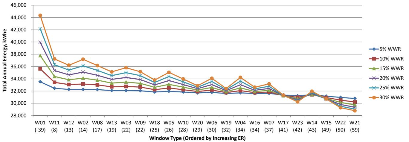
Fig.7.55 Total annual energy consumption for window to wall ratios in Winnipeg, kWh<sub>e</sub>.
