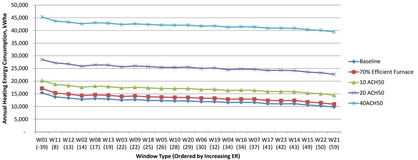
Fig.7.91 Annual heating energy consumption in Toronto, kWh<sub>e</sub>.
