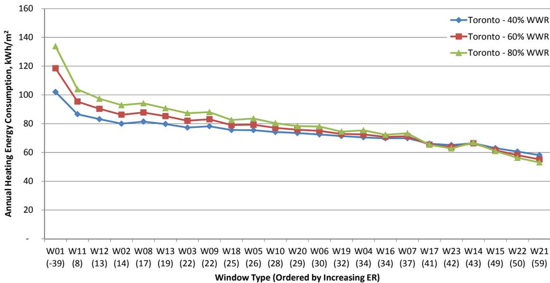
Fig.11.31 Annual heating energy consumption for high-rise building in Toronto, kWh<sub>e</sub>/m<sup>2</sup>.
