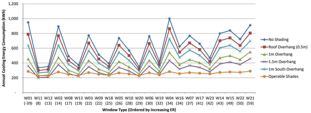
Fig.7.89 Annual cooling energy consumption for window shading scenarios in Yellowknife, kWh.
