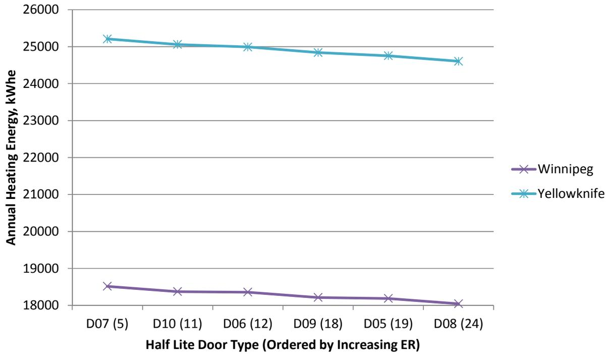
Fig.10.14 Annual heating energy consumption of half lite doors, Winnipeg and Yellowknife, kWh<sub>e</sub>.
