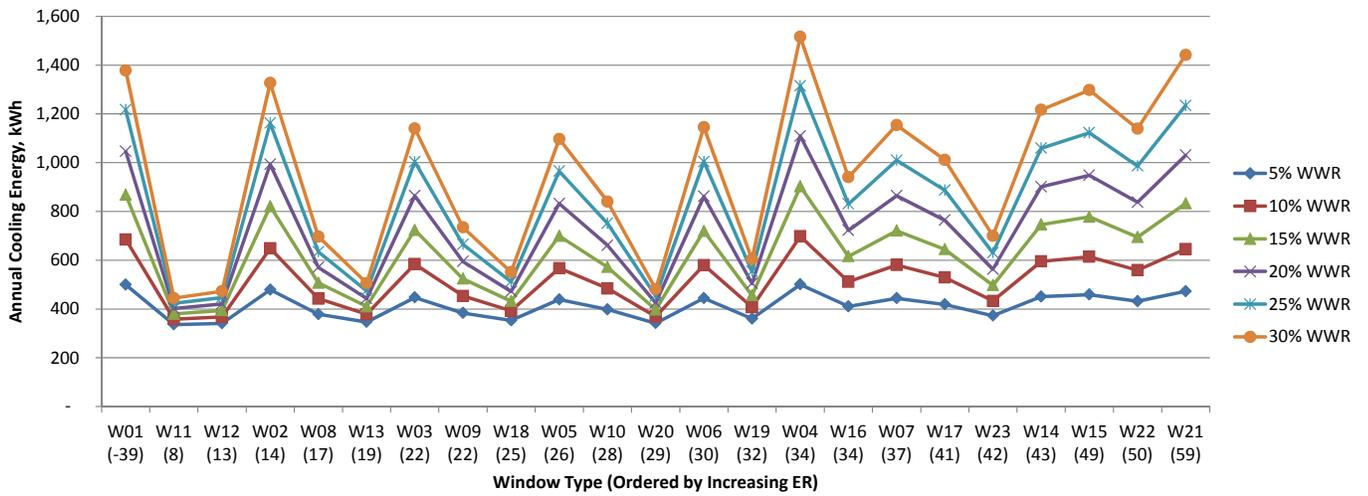
Fig.7.45 Annual cooling energy consumption for window to wall ratios in Vancouver, kWh.
