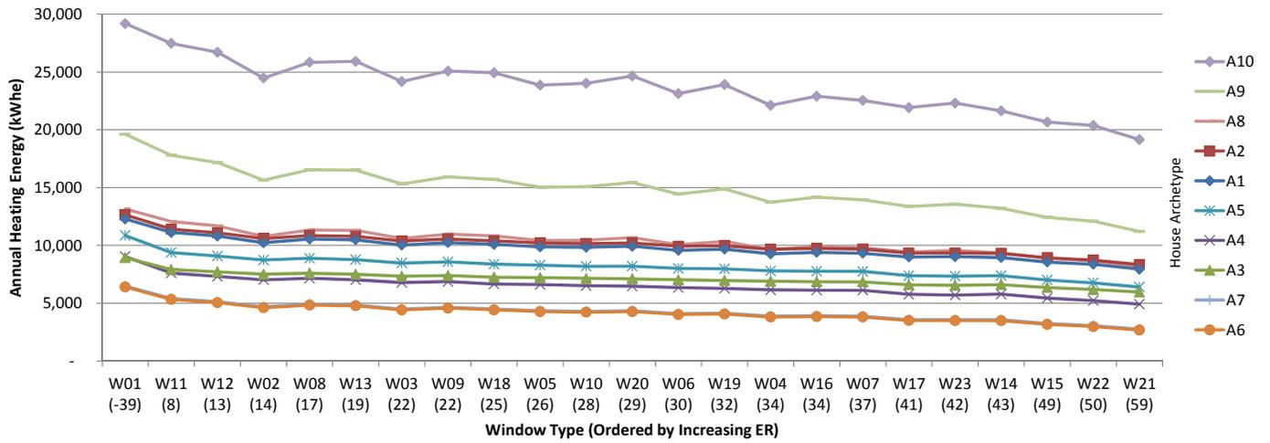
Fig.7.29 Annual heating energy consumption for archetype houses in Vancouver, kWh<sub>e</sub>.
