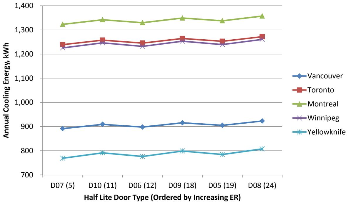
Fig.10.15 Annual cooling energy consumption of half lite doors, kWh.
