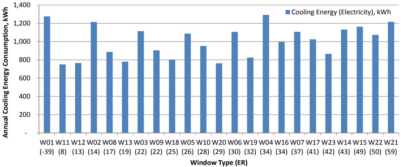
Fig.7.19 Annual cooling energy consumption in Toronto, kWh.
