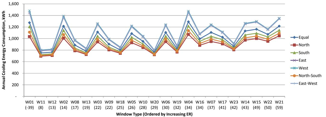
Fig.7.63 Annual cooling energy consumption for window orientations in Toronto, kWh.
