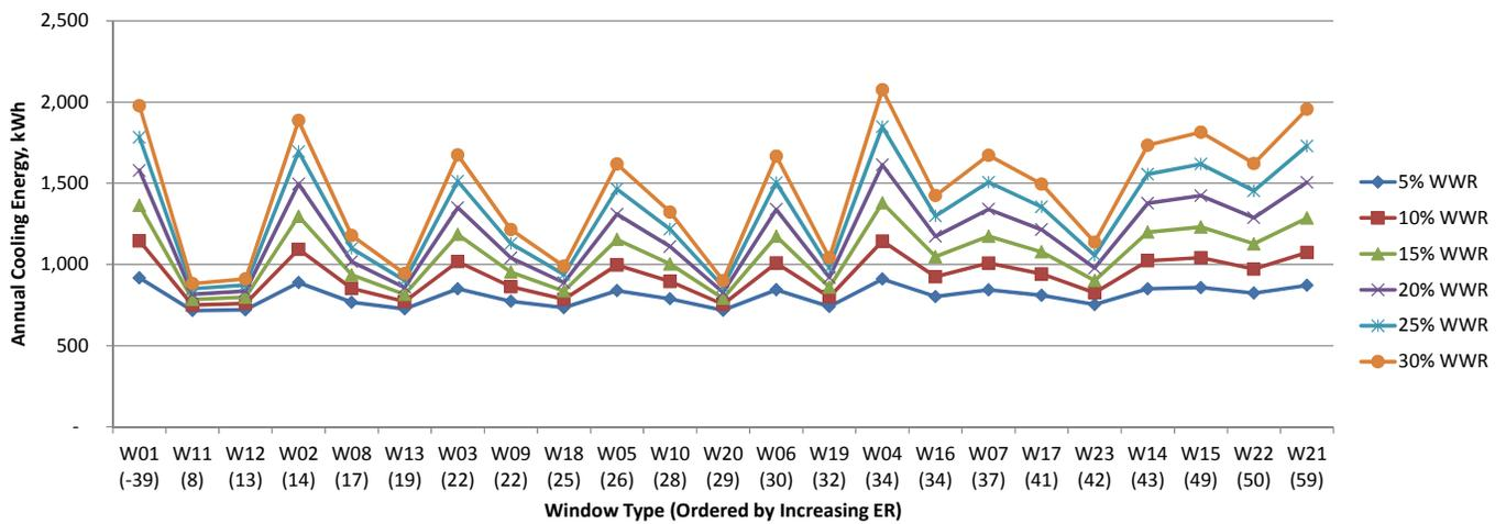
Fig.7.51 Annual cooling energy consumption for window to wall ratios in Montreal, kWh.
