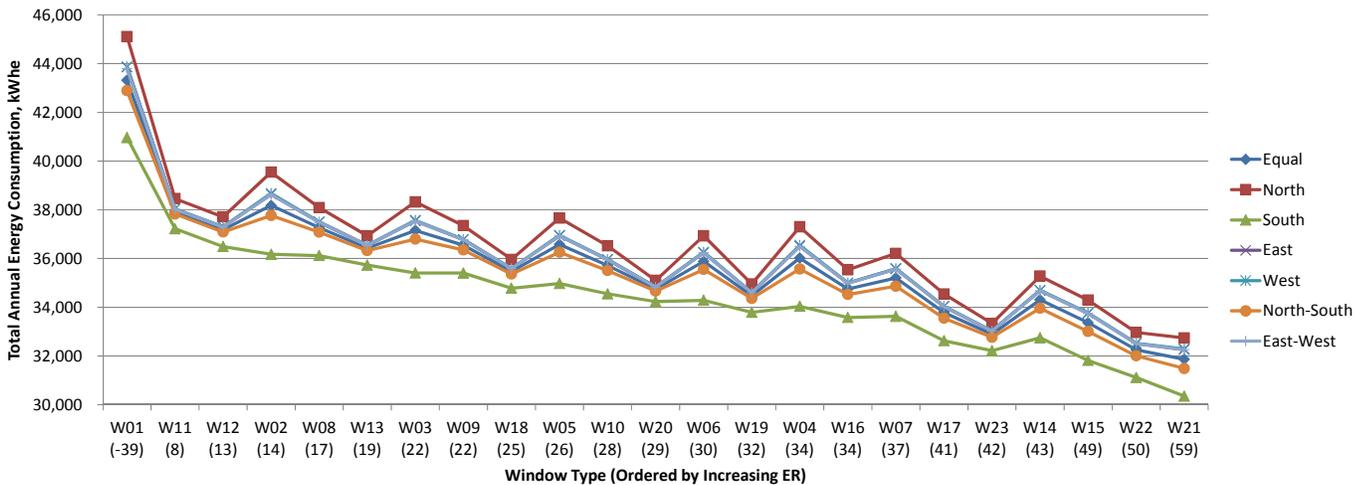
Fig.7.73 Total annual energy consumption for window orientations in Yellowknife, kWh<sub>e</sub>.
