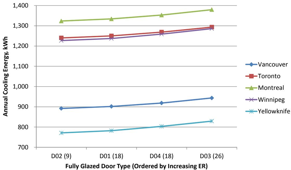
Fig.10.11 Annual cooling energy consumption of fully glazed doors, kWh.
