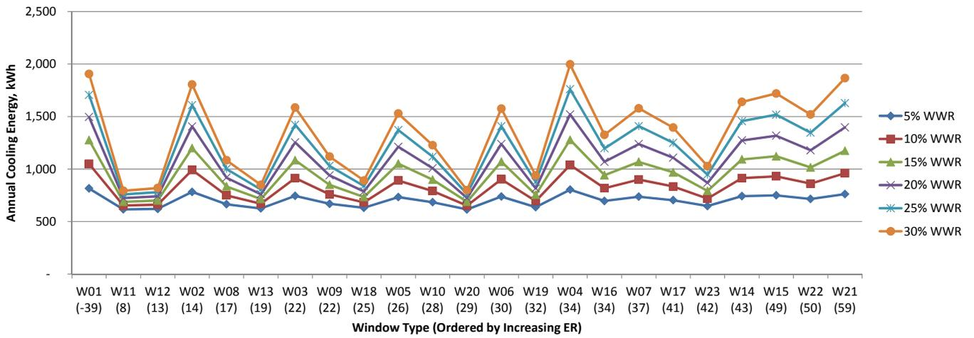
Fig.7.54 Annual cooling energy consumption for window to wall ratios in Winnipeg, kWh.
