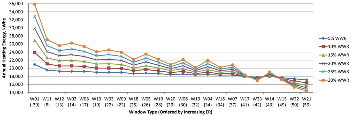
Fig.7.56 Annual heating energy consumption for window to wall ratios in Yellowknife, kWh<sub>e</sub>.
