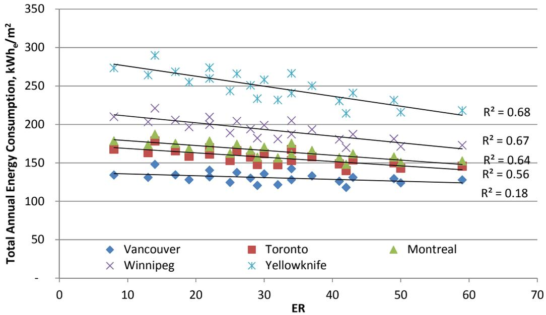
Fig.11.35 Total annual energy versus ER, 60% WWR, kWh<sub>e</sub>/m<sup>2</sup>.
