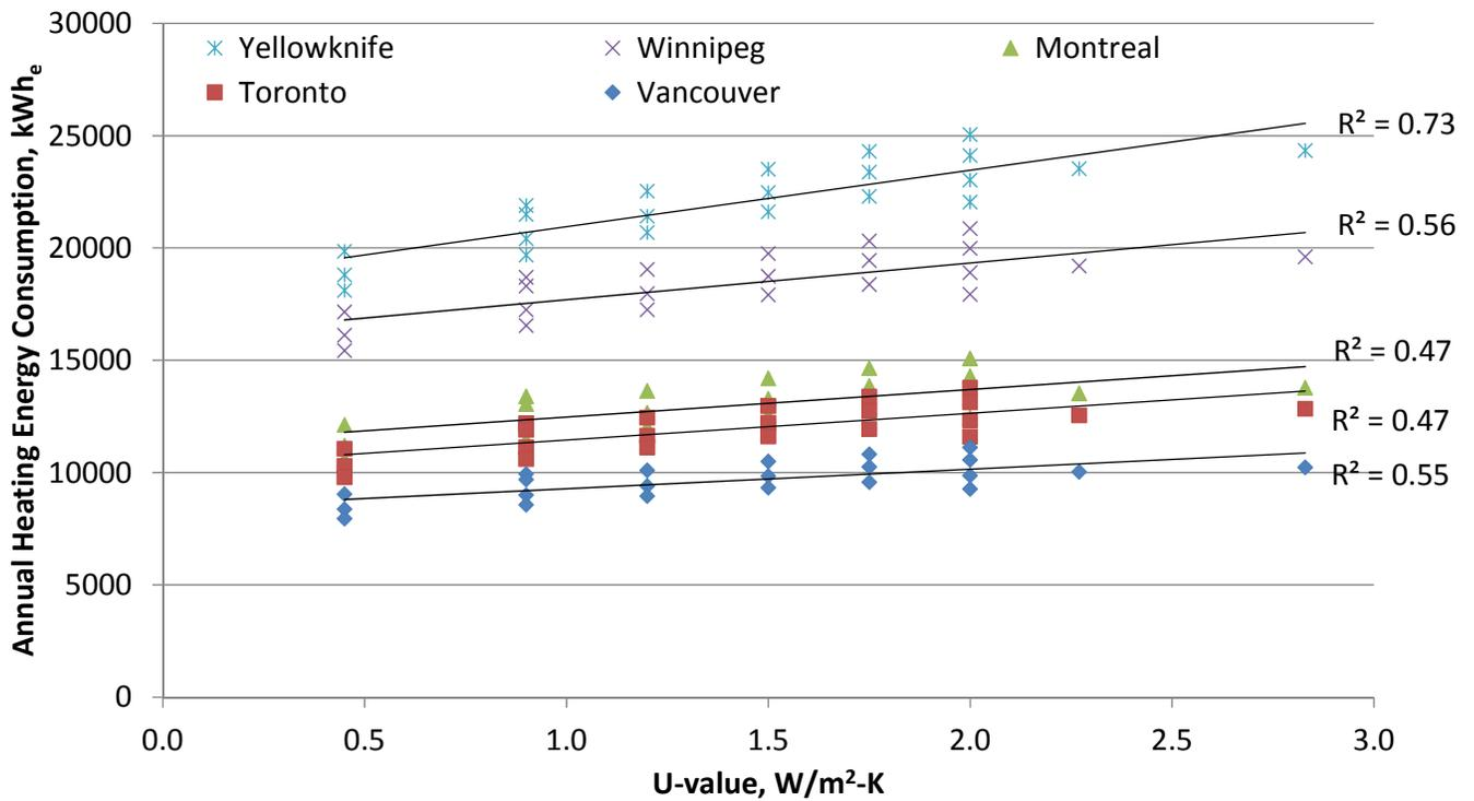
Fig.7.28 Heating energy consumption versus U-value.
