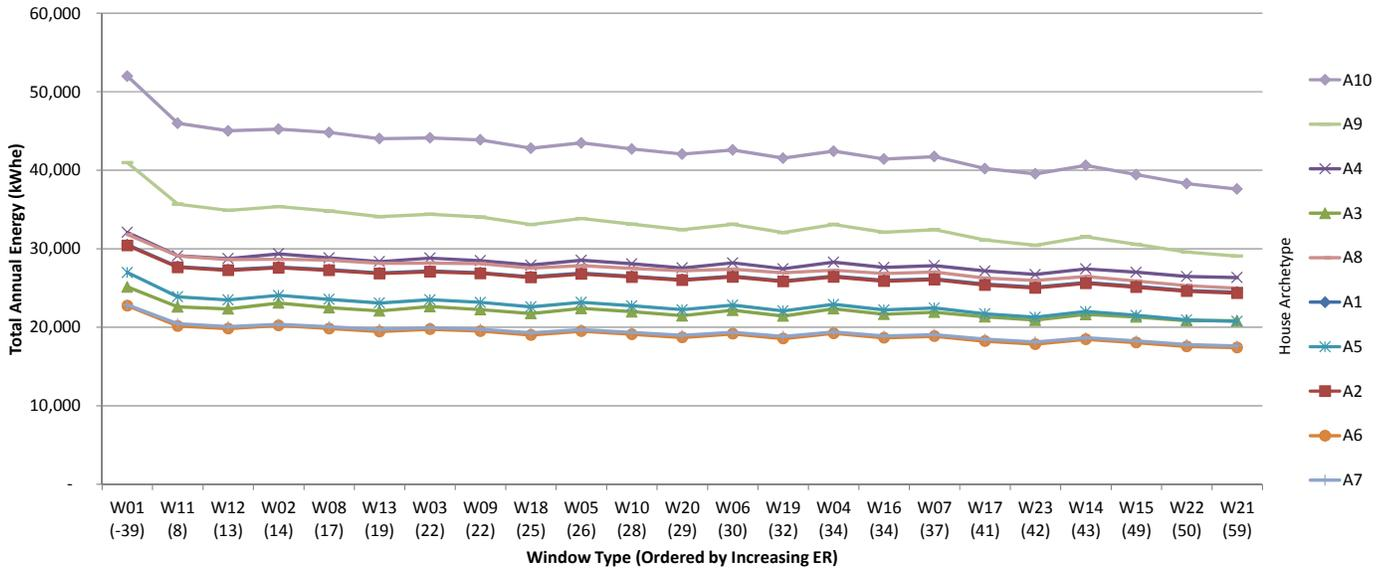
Fig.7.34 Total annual energy consumption for archetype houses in Toronto, kWh<sub>e</sub>.
