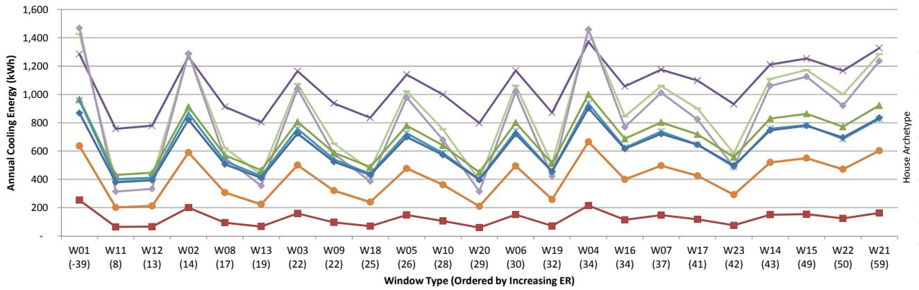
Fig.7.30 Annual cooling energy consumption for archetype houses in Vancouver, kWh.
