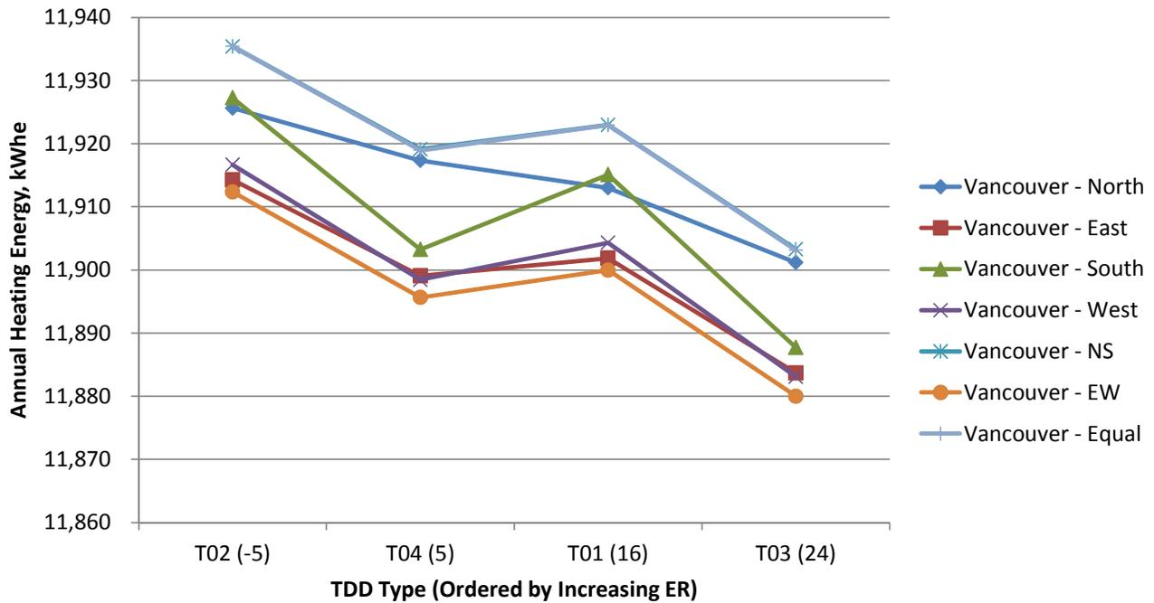
Fig.10.28 Annual heating energy consumption, Vancouver, kWh<sub>e</sub>.
