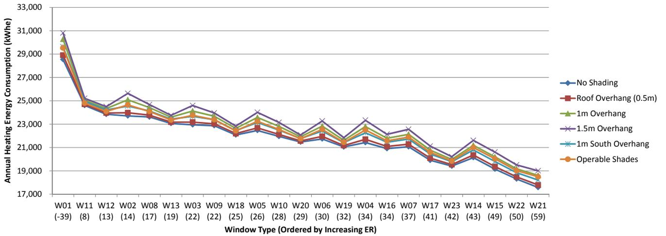
Fig.7.88 Annual heating energy consumption for window shading scenarios in Yellowknife, kWh<sub>e</sub>.
