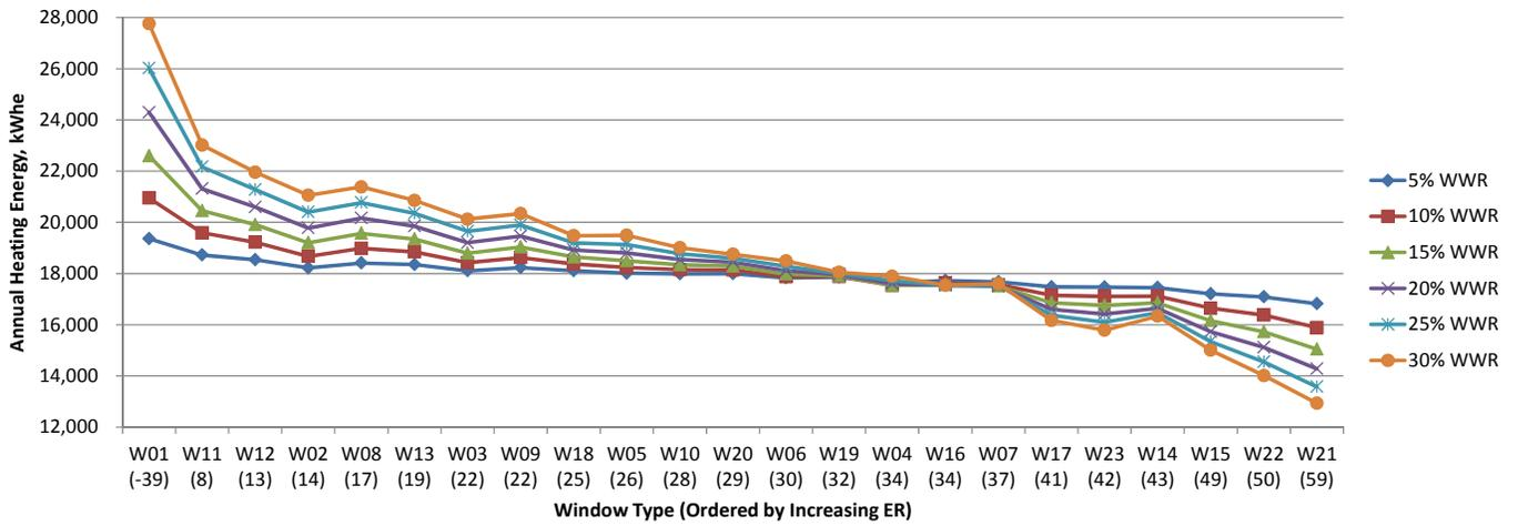
Fig.7.53 Annual heating energy consumption for window to wall ratios in Winnipeg, kWh<sub>e</sub>.
