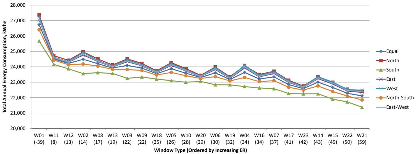
Fig.7.61 Total annual energy consumption for window orientations in Vancouver, kWh<sub>e</sub>.
