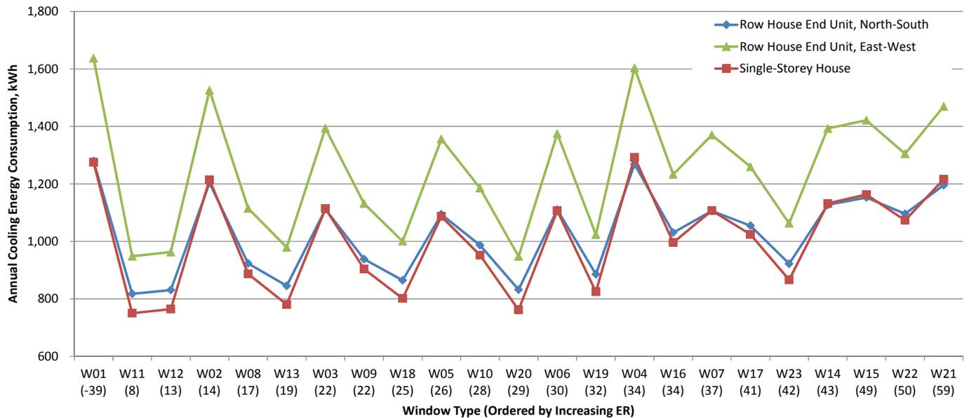
Fig.11.11 Annual cooling energy consumption, row house and single-storey archetypes in Toronto, kWh.
