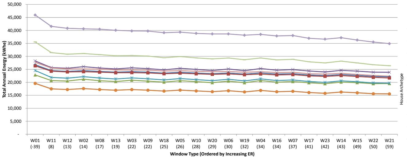
Fig.7.31 Total annual energy consumption for archetype houses in Vancouver, kWh<sub>e</sub>.
