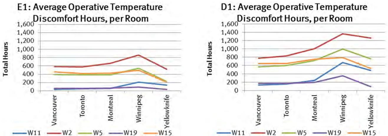
Fig. 9.5.32 E1, Operative temperature discomfort hours per room compared with D1
