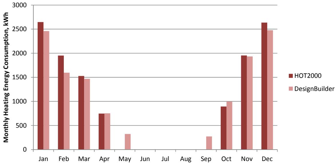
Fig.7.9 Monthly heating energy simulated in HOT2000 and DesignBuilder in Vancouver.
