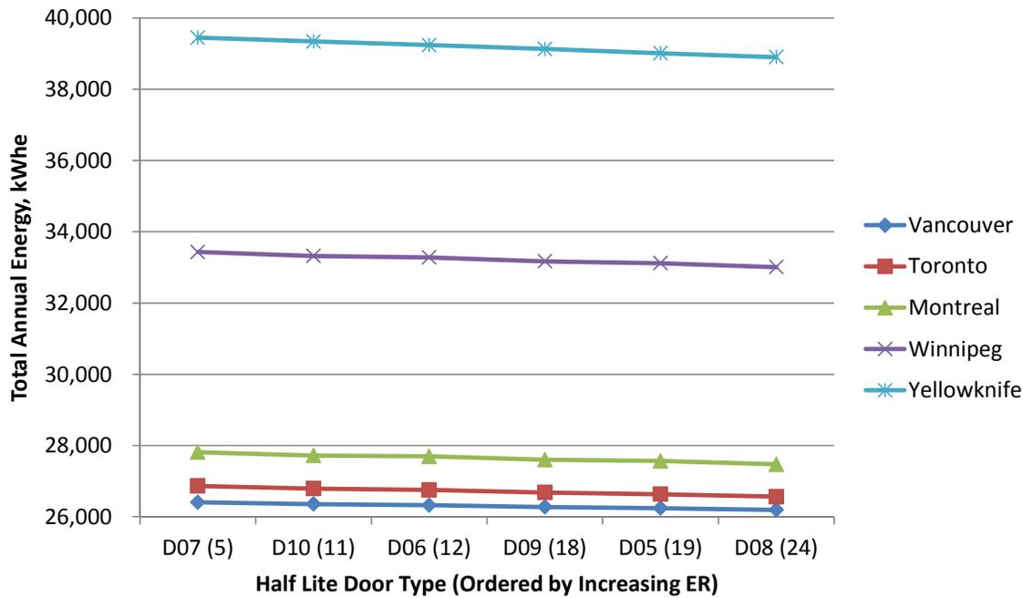
Fig.10.16 Total annual energy consumption of half lite doors, kWh<sub>e</sub>.
