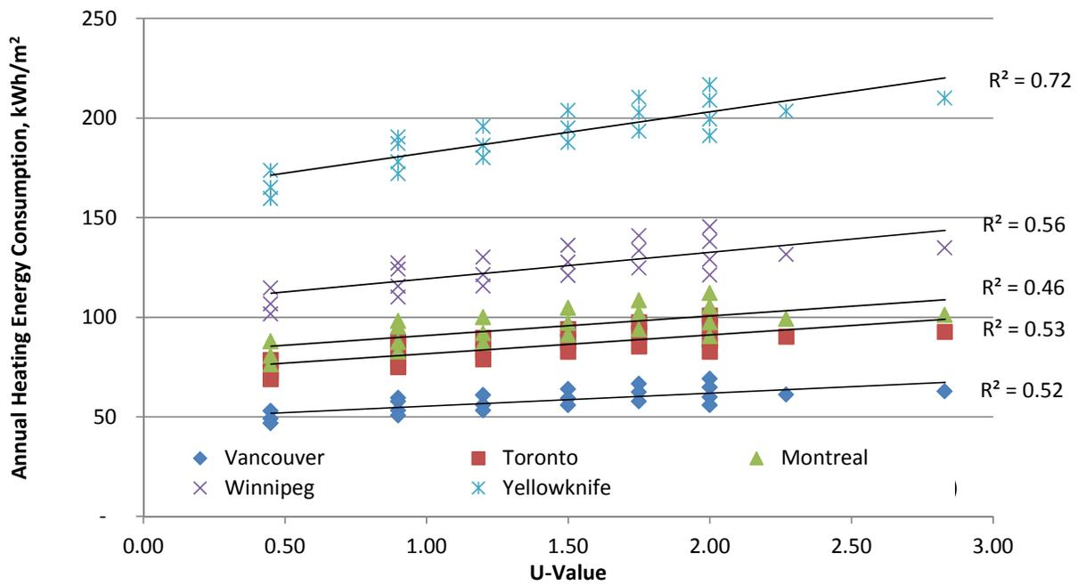
Fig.11.23 Annual heating energy consumption versus U-value, 40% WWR, kWh/m<sup>2</sup>.
