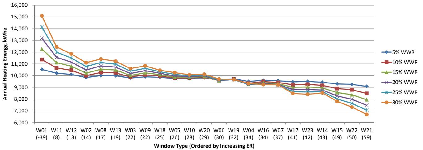
Fig.7.44 Annual heating energy consumption for window to wall ratios in Vancouver, kWh<sub>e</sub>.
