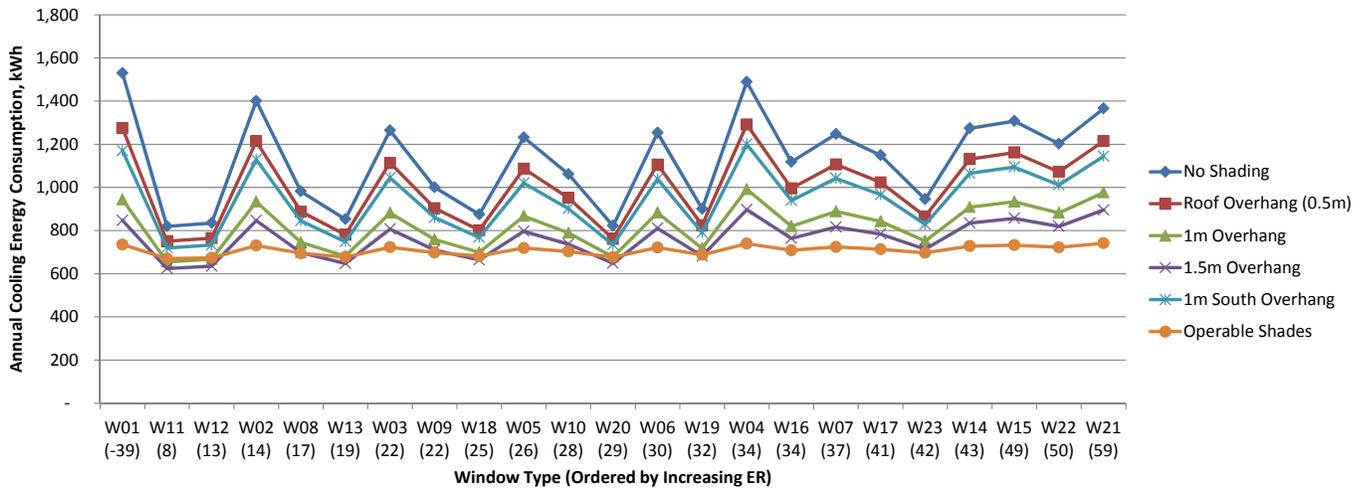
Fig.7.80 Annual cooling energy consumption for window shading scenarios in Toronto, kWh.
