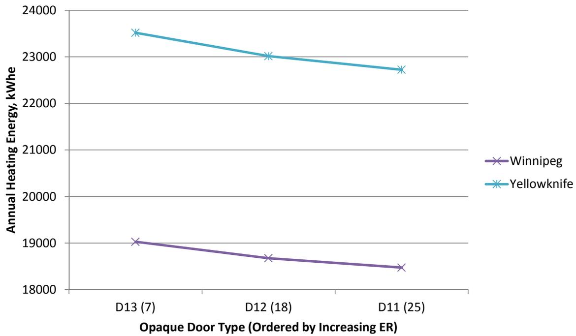
Fig.10.18 Annual heating energy consumption of half lite doors, Winnipeg and Yellowknife, kWh<sub>e</sub>.
