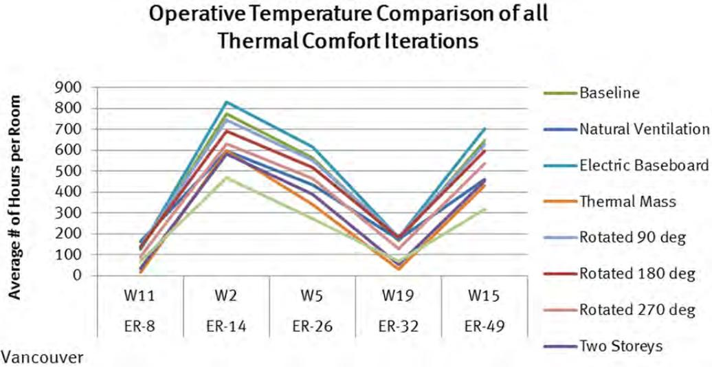
Fig. 9.4.33 Vancouver, All iterations operative temperature discomfort hours
