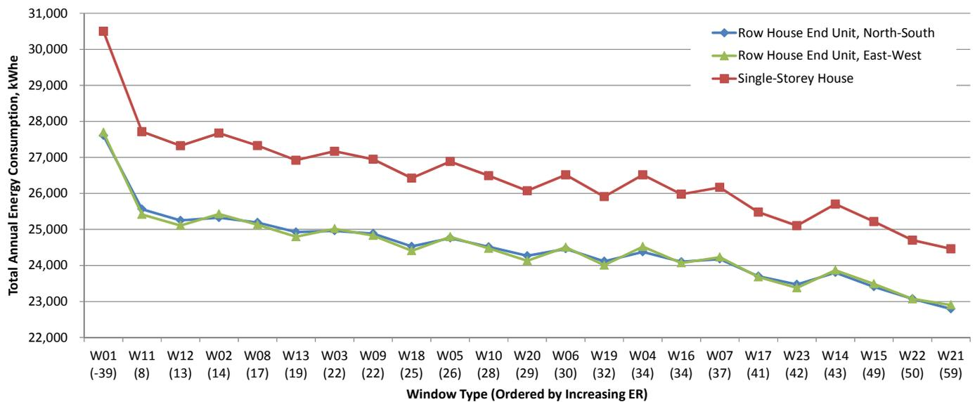
Fig.11.12 Total annual energy consumption, row house and single-storey archetypes in Toronto, kWh<sub>e</sub>.
