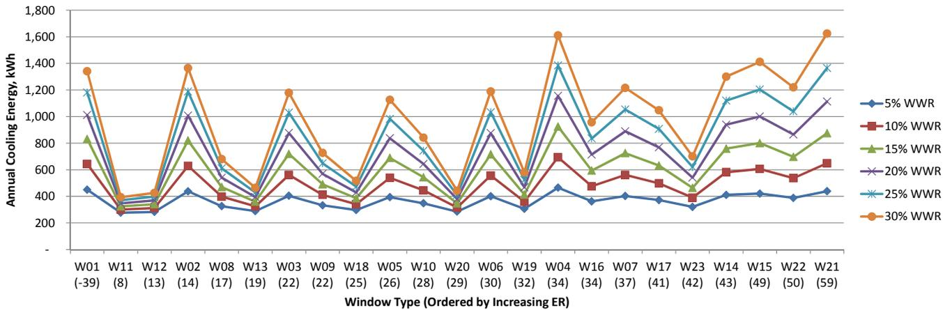
Fig.7.57 Annual cooling energy consumption for window to wall ratios in Yellowknife, kWh.
