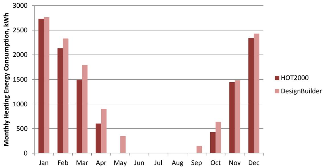
Fig.7.11 Monthly heating energy simulated in HOT2000 and DesignBuilder in Toronto.
