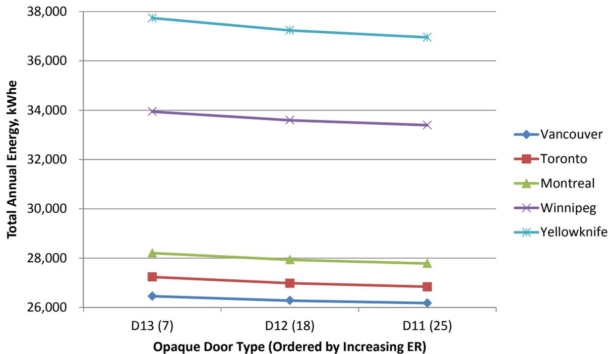
Fig.10.20 Total annual energy consumption of opaque doors, kWh<sub>e</sub>.
