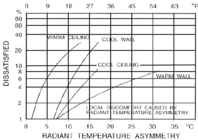
Fig. 9.3.6 ASHRAE Standard 55-2010 (Fig 5.2.4.1), Allowable radiant asymmetry
