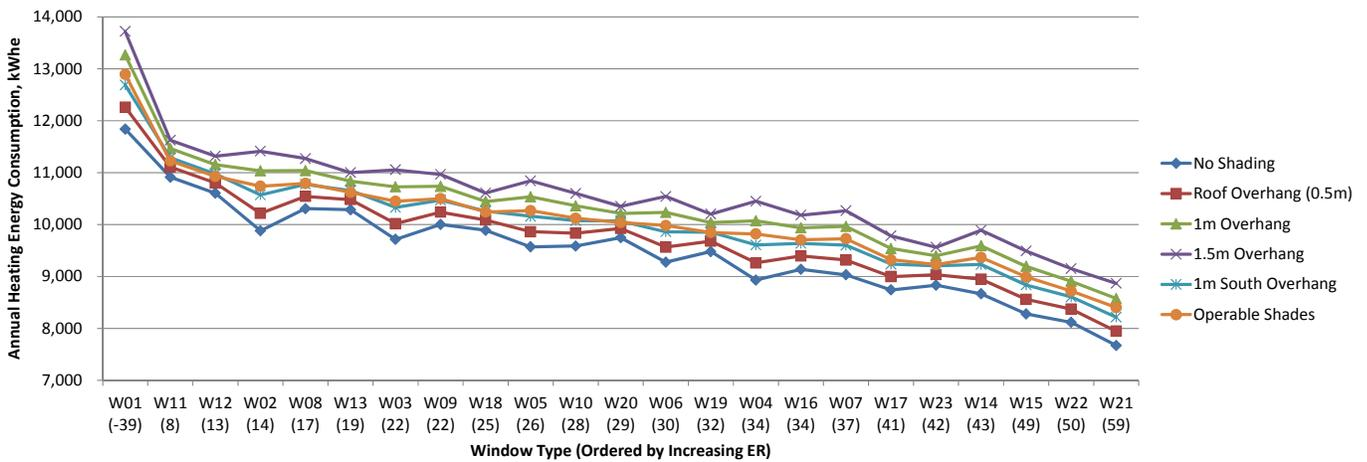
Fig.7.76 Annual heating energy consumption for window shading scenarios in Vancouver, kWh<sub>e</sub>.
