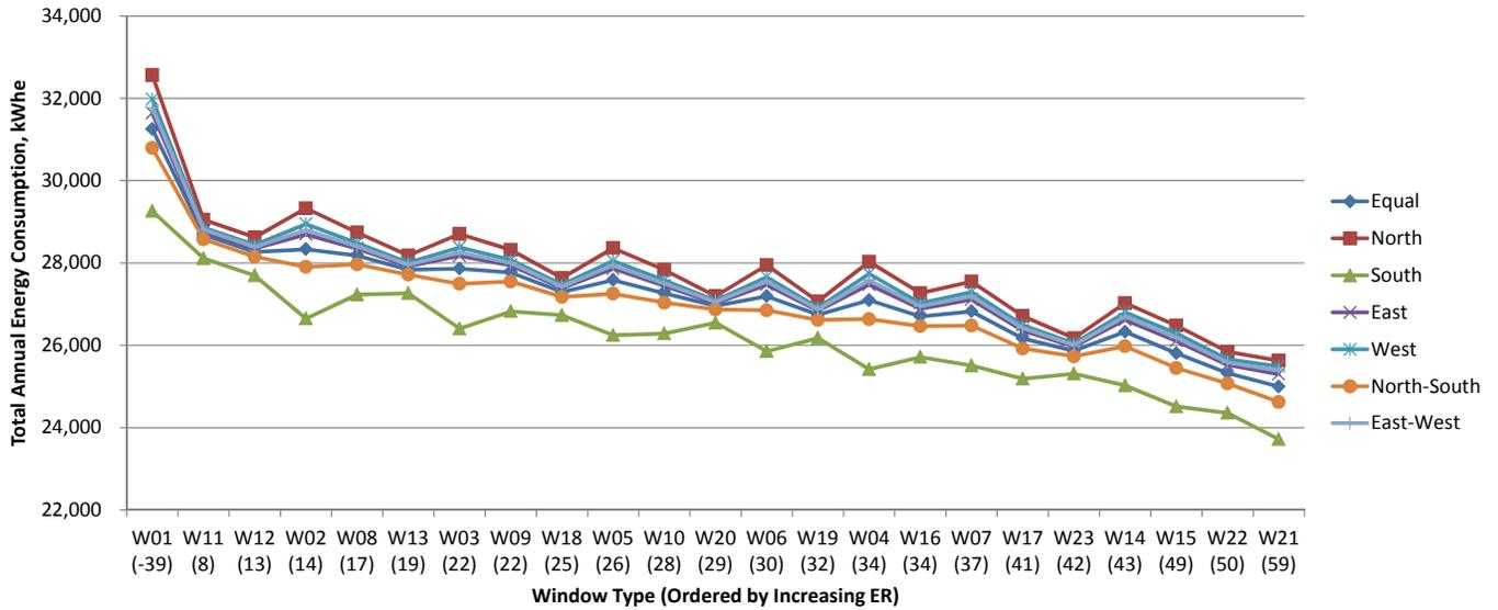
Fig.7.67 Total annual energy consumption for window orientations in Montreal, kWh<sub>e</sub>.
