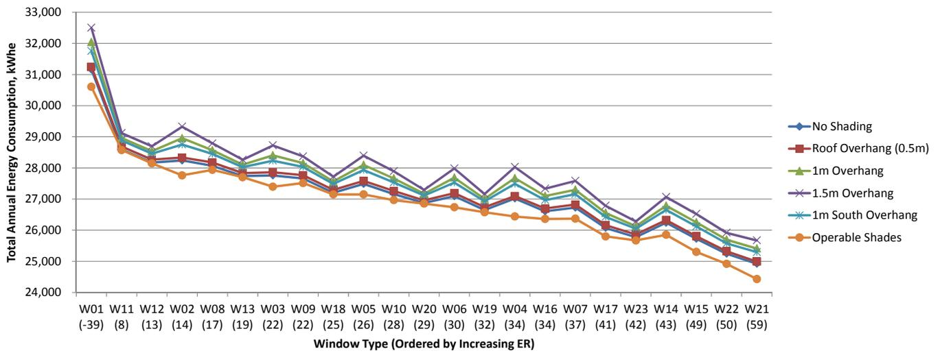
Fig.7.84 Total annual energy consumption for window shading scenarios in Montreal, kWh<sub>e</sub>.
