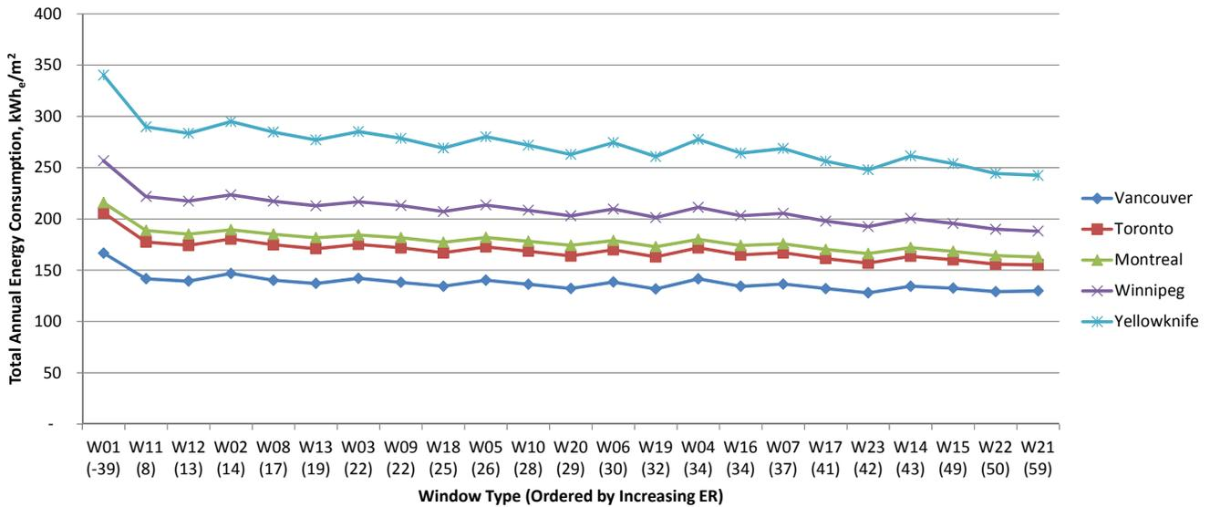
Fig.11.17 Total annual energy consumption for low-rise building with 40% WWR, kWh<sub>e</sub>/m<sup>2</sup>.
