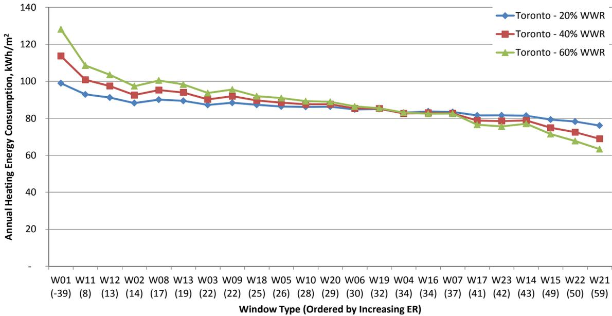
Fig.11.18 Annual heating energy consumption for low-rise building in Toronto, kWh/m<sup>2</sup>.
