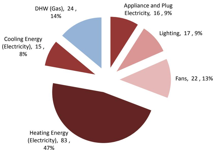
Fig.11.26 Distribution of high-rise building energy consumption in Vancouver, 60% WWR, kWh<sub>e</sub>/m<sup>2</sup> and percent of total.
