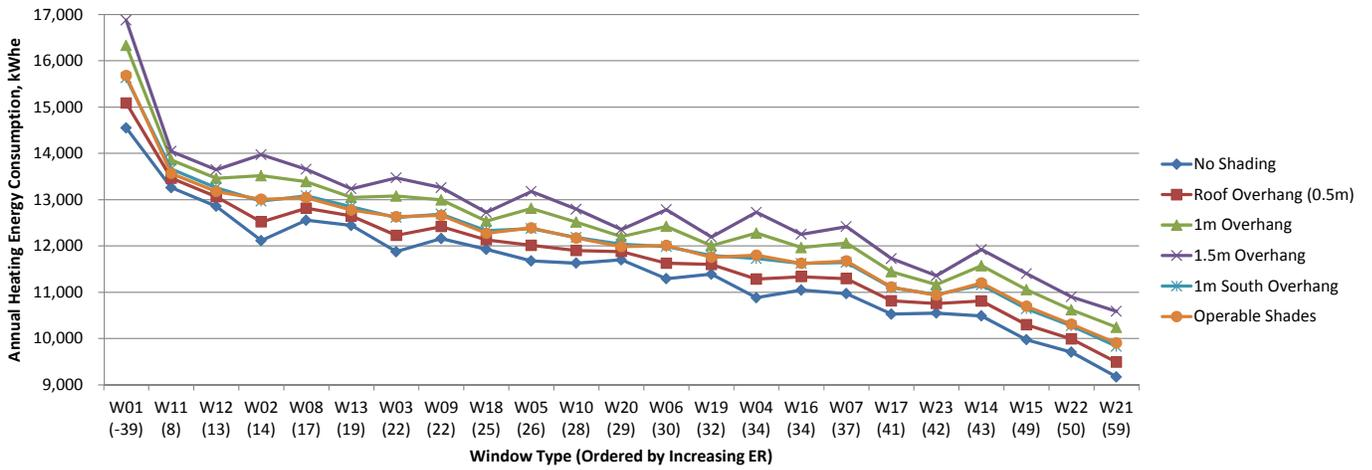
Fig.7.79 Annual heating energy consumption for window shading scenarios in Toronto, kWh<sub>e</sub>.
