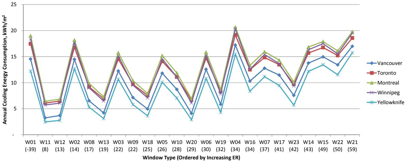
Fig.11.29 Annual cooling energy consumption for high-rise building with 60% WWR, kWh/m<sup>2</sup>.
