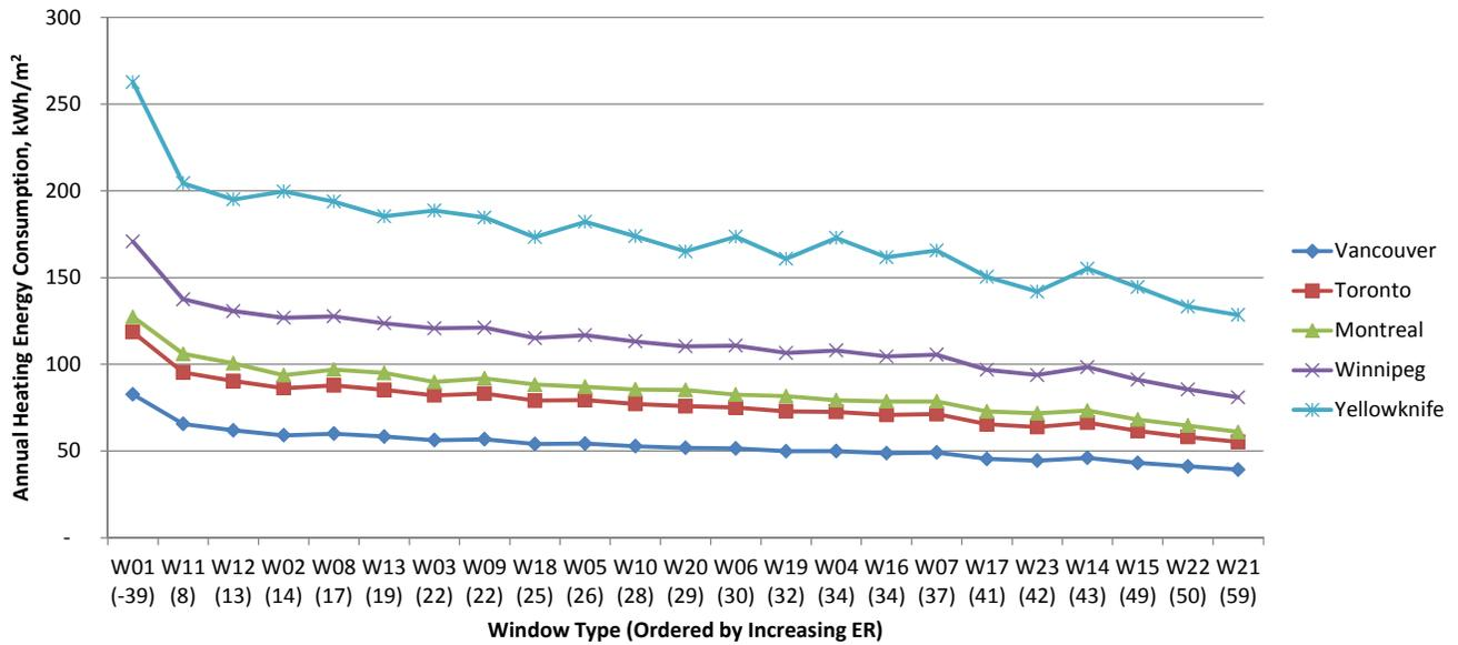
Fig.11.28 Annual heating energy consumption for high-rise building with 60% WWR, kWh/m<sup>2</sup>.
