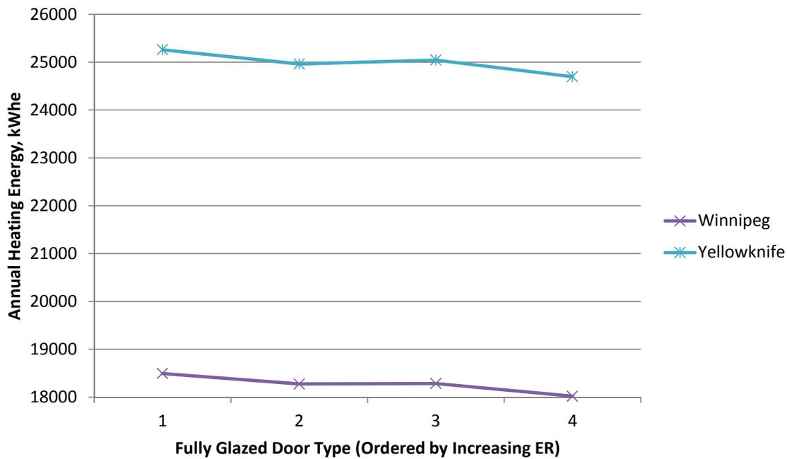
Fig.10.10 Annual heating energy consumption of fully glazed doors, Winnipeg and Yellowknife, kWh<sub>e</sub>.
