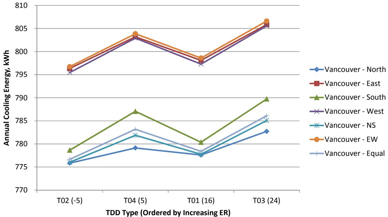
Fig.10.29 Annual cooling energy consumption, Vancouver, kWh.
