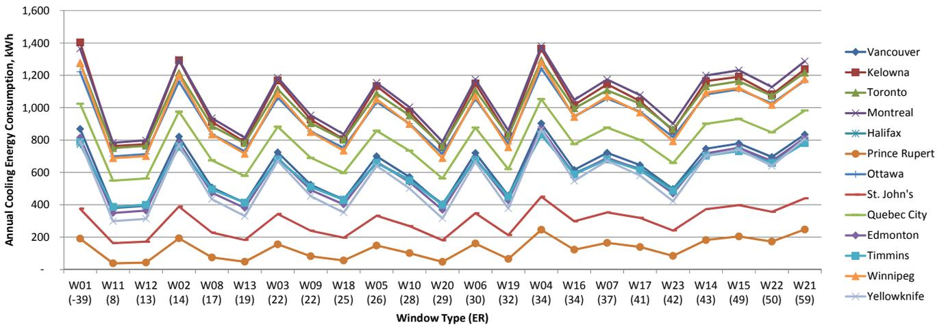
Fig.7.25 Annual cooling energy consumption, kWh.
