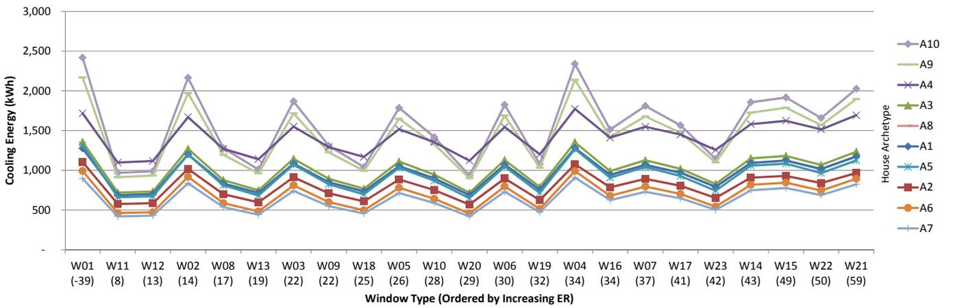
Fig.7.39 Annual cooling energy consumption for archetype houses in Winnipeg, kWh.
