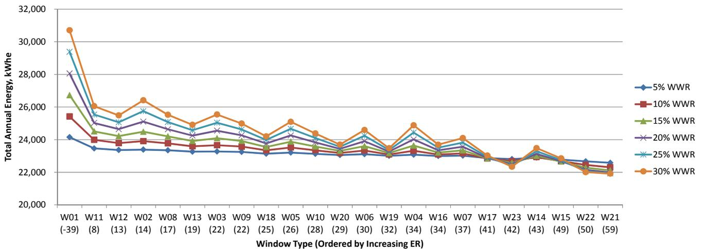
Fig.7.46 Total annual energy consumption for window to wall ratios in Vancouver, kWh<sub>e</sub>.
