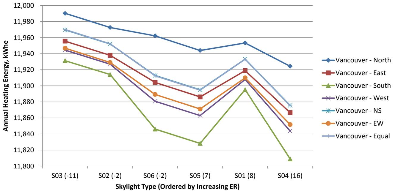
Fig.10.24 Annual heating energy consumption, Vancouver, kWh<sub>e</sub>.
