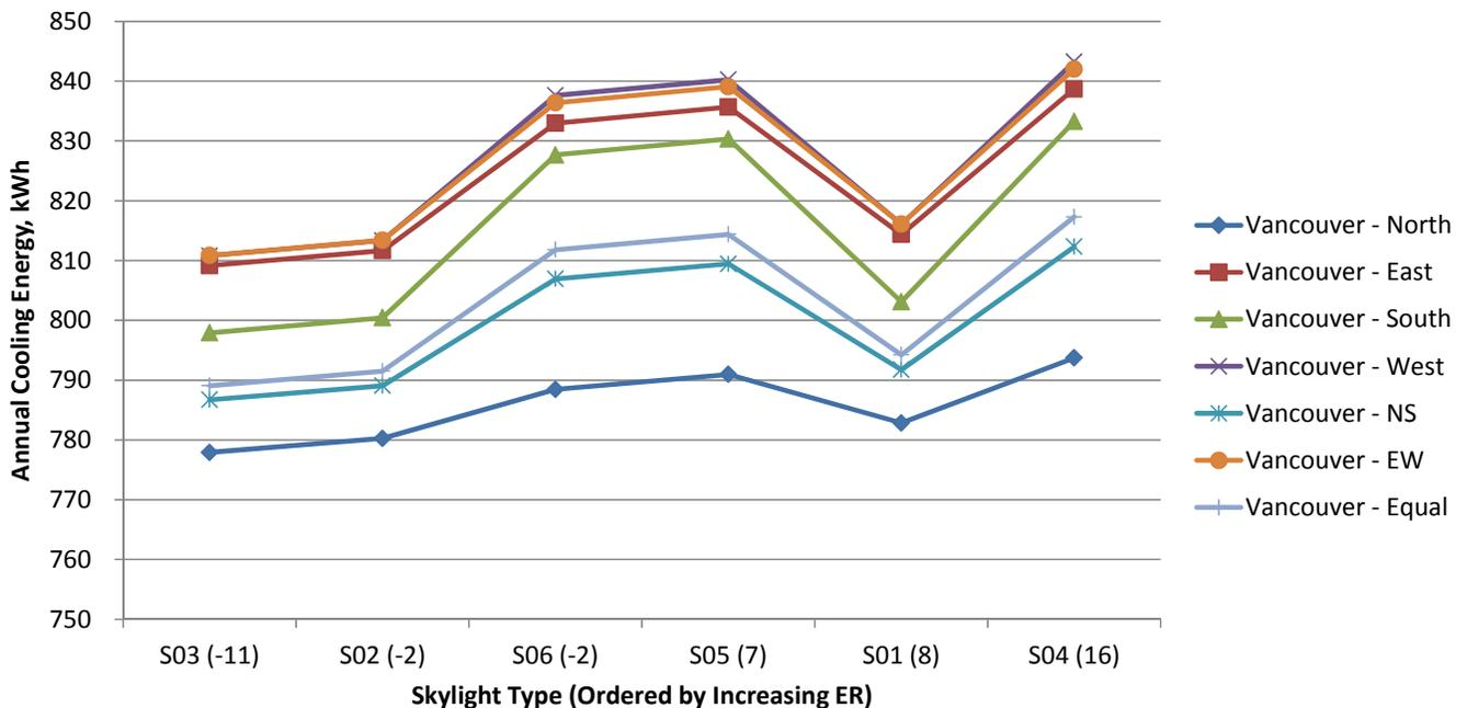
Fig.10.25 Annual cooling energy consumption, Vancouver, kWh.
