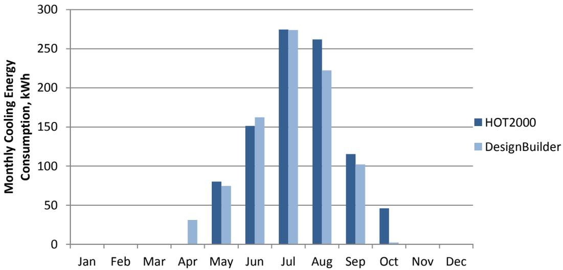
Fig.7.10 Monthly cooling energy simulated in HOT2000 and DesignBuilder in Vancouver.
