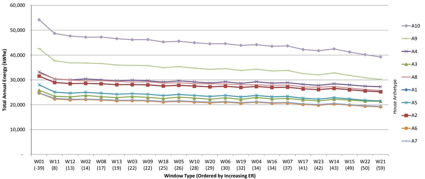
Fig.7.37 Total annual energy consumption for archetype houses in Montreal, kWh<sub>e</sub>.
