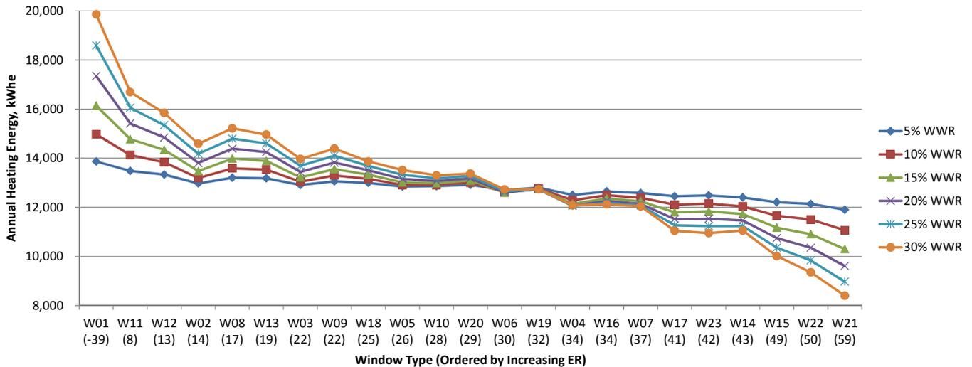
Fig. 7.50 Annual heating energy consumption for window to wall ratios in Montreal, kWh<sub>e</sub>.
