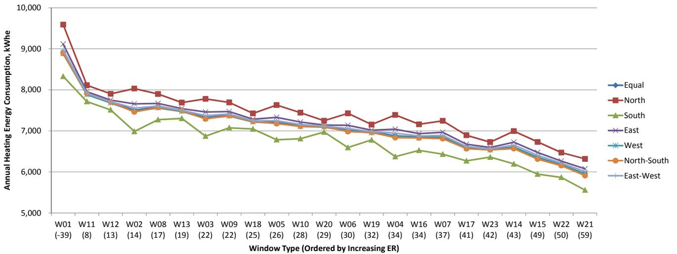
Fig.7.74 Annual heating energy consumption for window orientations in Vancouver with electric baseboard heating, kWh<sub>e</sub>.
