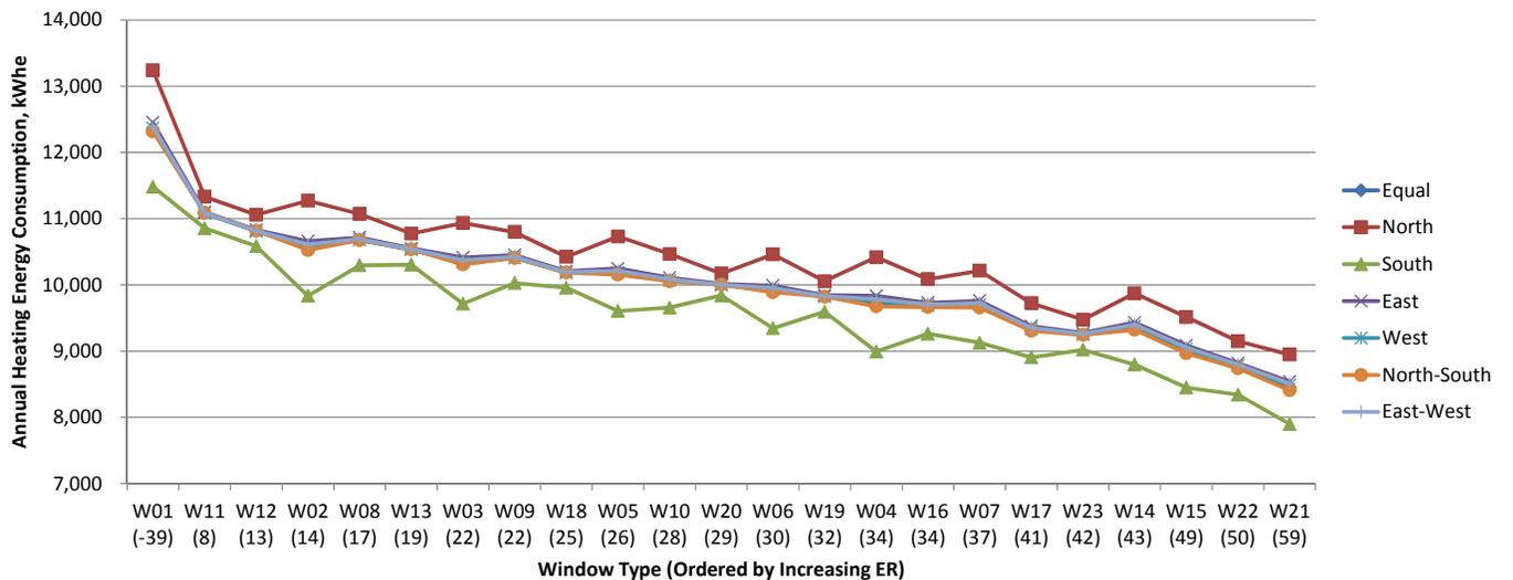
Fig.7.75 Annual heating energy consumption for window orientations in Toronto with electric baseboard heating, kWh<sub>e</sub>.
