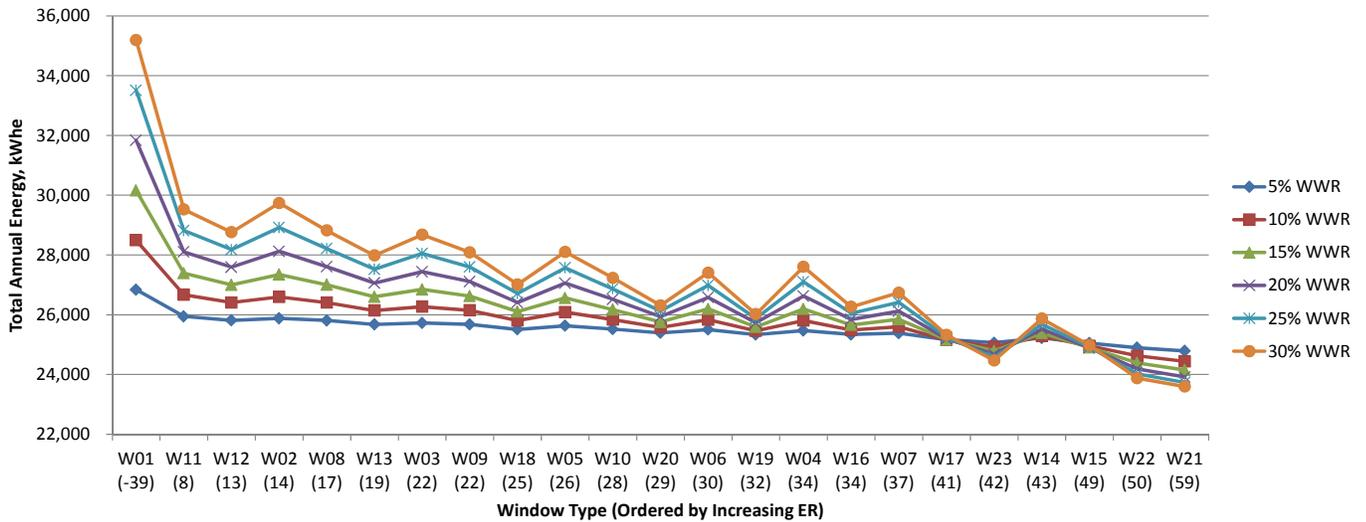
Fig. 7.49 Total annual energy consumption for window to wall ratios in Toronto, kWh<sub>e</sub>.
