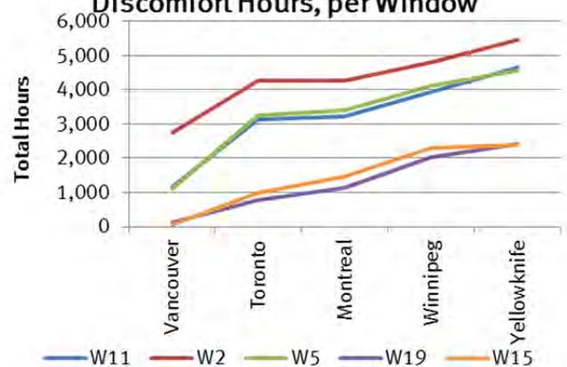
Fig. 9.5.43 E2, Average window surface temperature discomfort hours compared with D2
