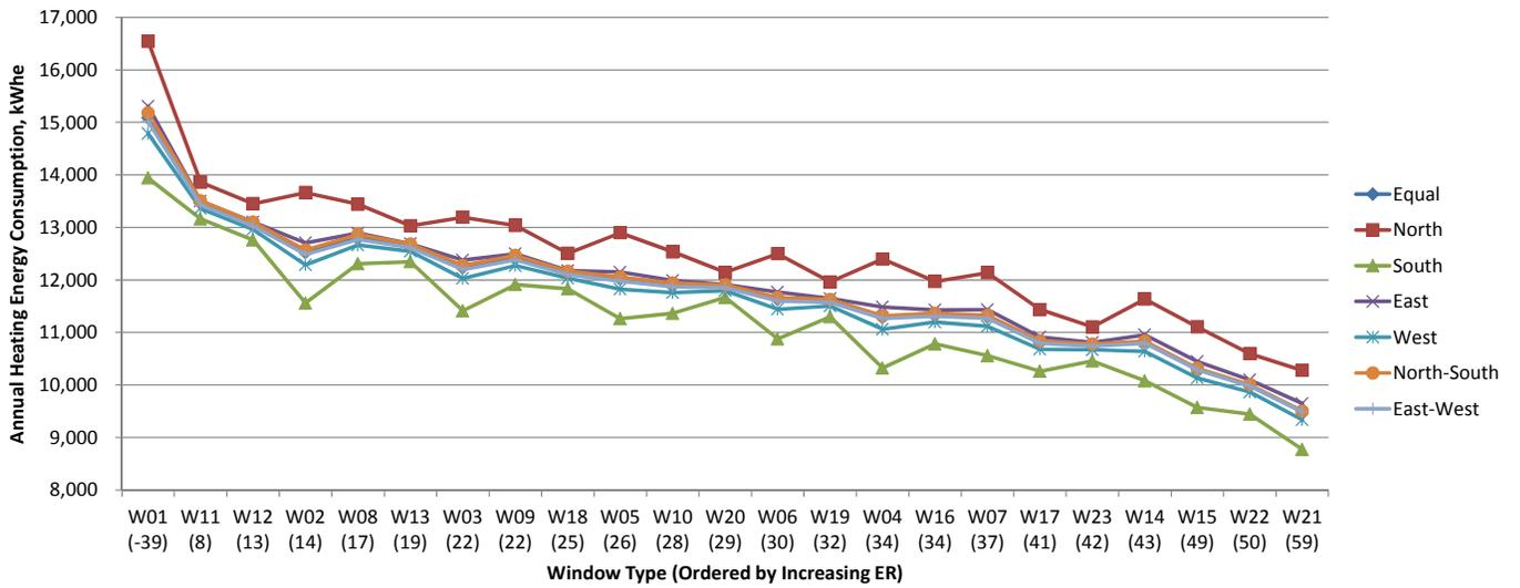
Fig.7.62 Annual heating energy consumption for window orientations in Toronto, kWh<sub>e</sub>.
