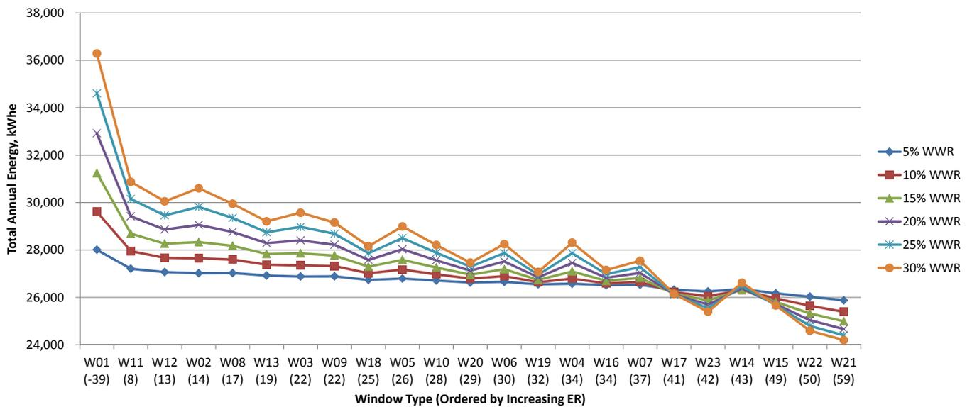
Fig.7.52 Total annual energy consumption for window to wall ratios in Montreal, kWh<sub>e</sub>.
