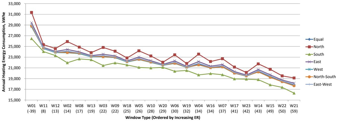
Fig.7.71 Annual heating energy consumption for window orientations in Yellowknife, kWh<sub>e</sub>.
