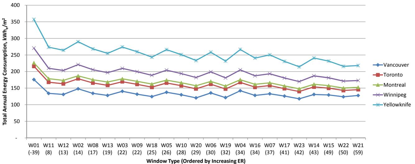
Fig.11.30 Total annual energy consumption for high-rise building with 60% WWR, kWh<sub>e</sub>/m<sup>2</sup>.
