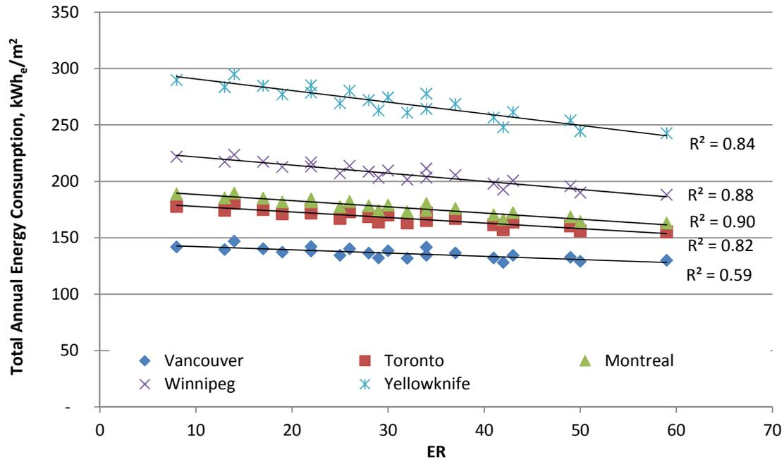
Fig.11.22 Total annual energy consumption versus ER, 40% WWR, kWh<sub>e</sub>/m<sup>2</sup>.
