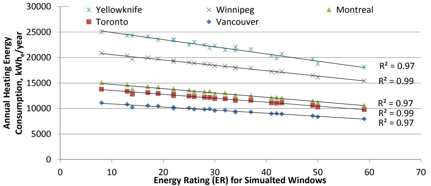
Fig.7.27 Heating energy consumption versus Energy Rating.
