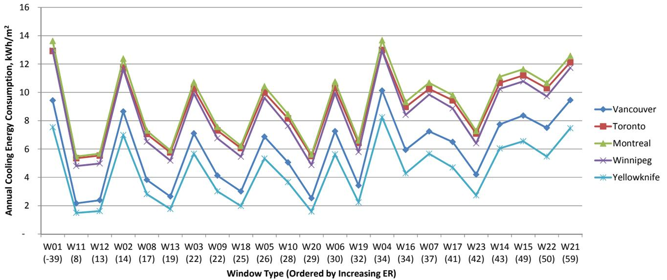
Fig.11.16 Annual cooling energy consumption for low-rise building with 40% WWR, kWh/m<sup>2</sup>.
