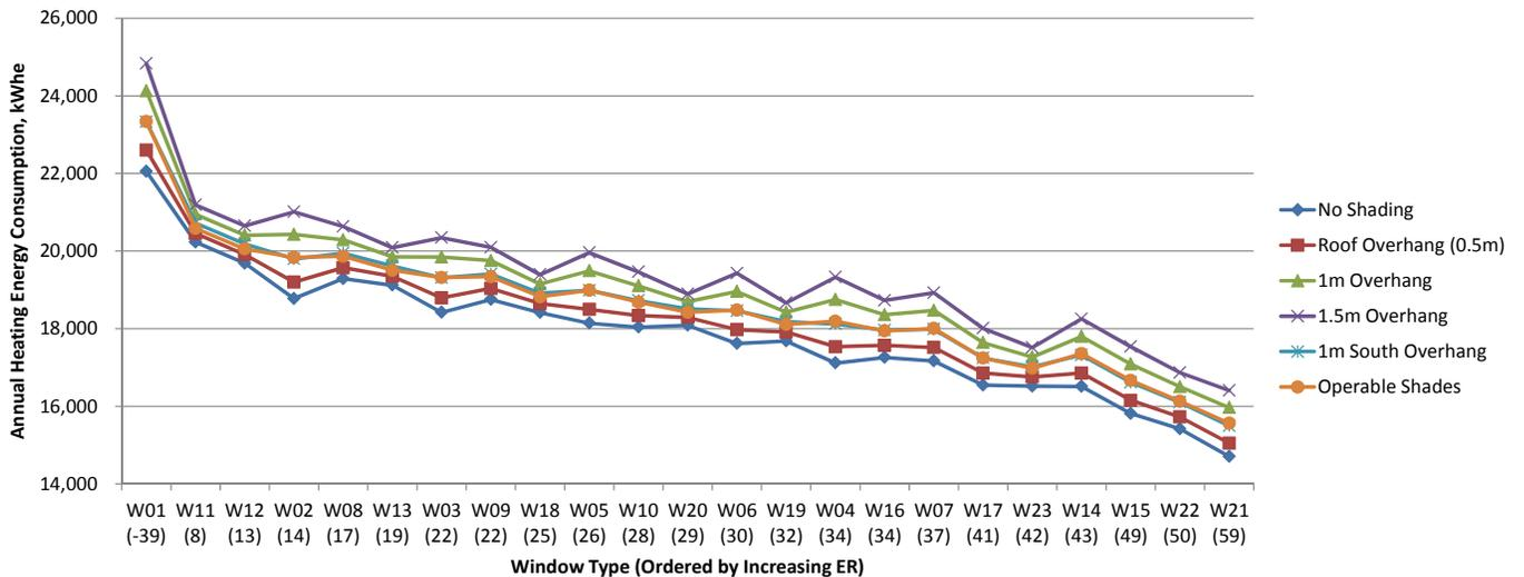
Fig.7.85 Annual heating energy consumption for window shading scenarios in Winnipeg, kWh<sub>e</sub>.
