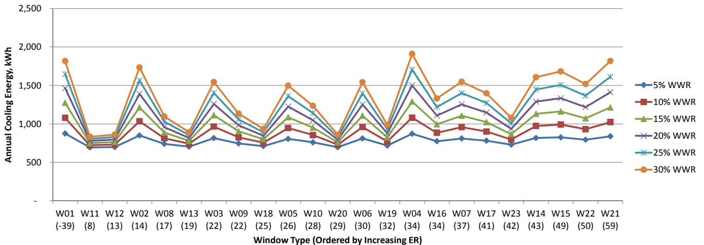
Fig.7.48 Annual cooling energy consumption for window to wall ratios in Toronto, kWh.
