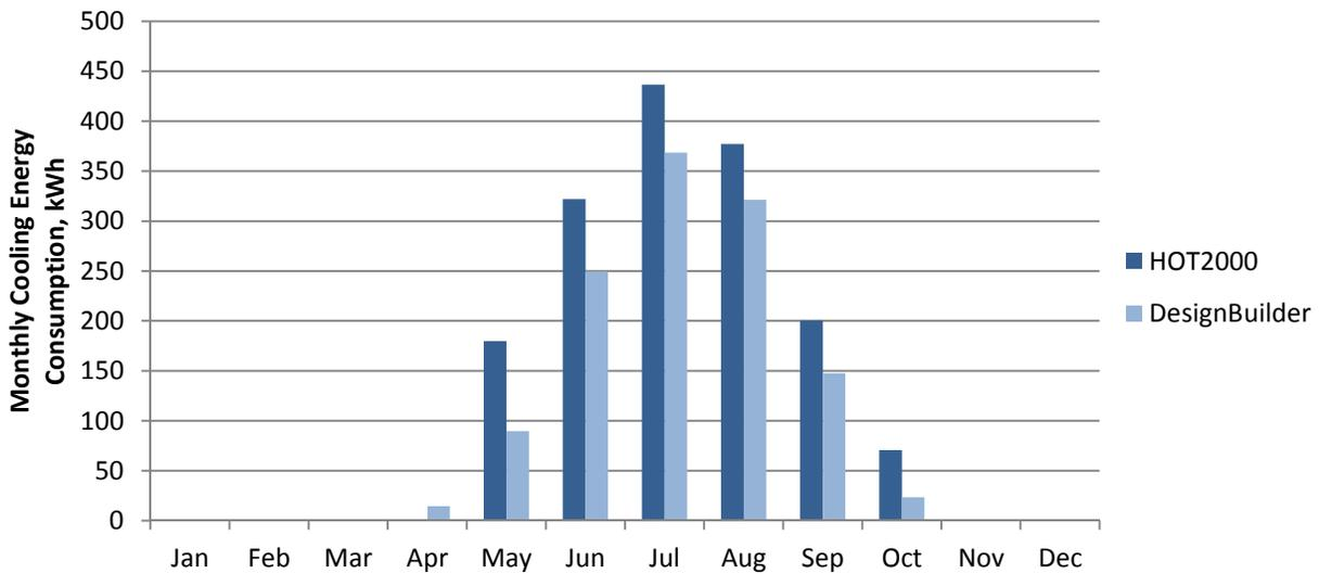
Fig.7.12 Monthly cooling energy simulated in HOT2000 and DesignBuilder in Toronto.
