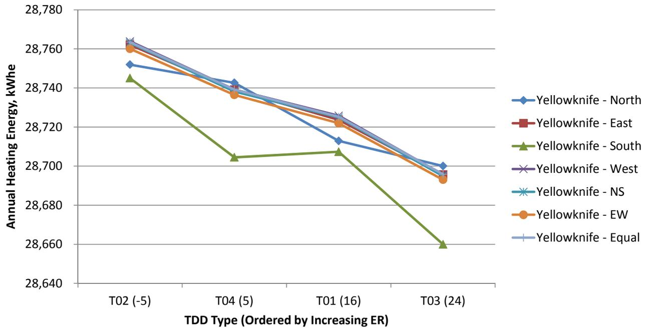
Fig.10.31 Annual heating energy consumption, Yellowknife, kWh<sub>e</sub>.
