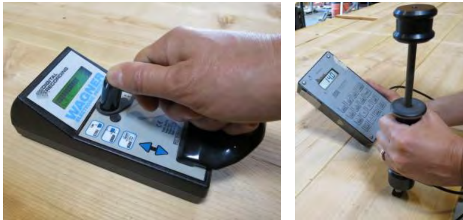
Figure 3 Measuring wood moisture content using a capacitance-based meter (left) and a resistance-based meter (right)
