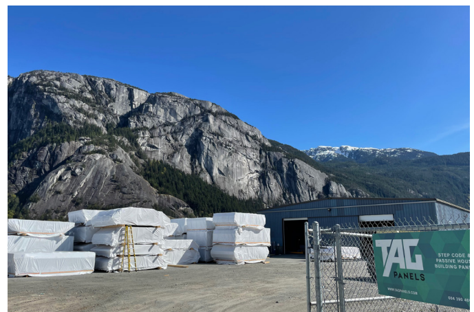
Figure 8. Panels stored inside protective coverings at the manufacturer (source: Scius)
