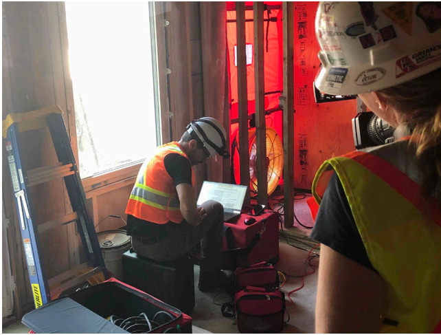
Multivista provided video documentation of the blower door test. (Source: Scius)
