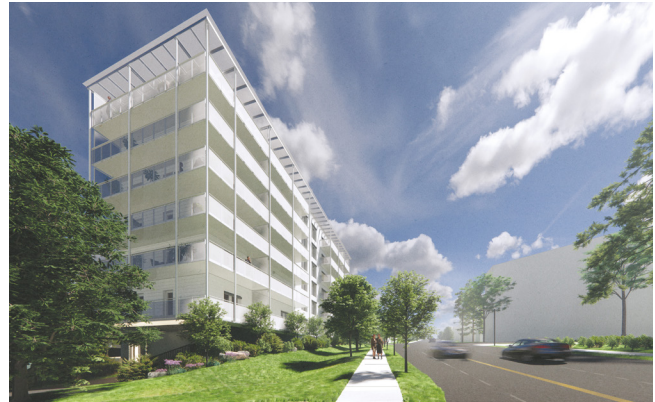
Figure 10. Illustration of the south-facing balconies for Vienna House with thermal break at connection (source: Sapphire Balconies Ltd.).
