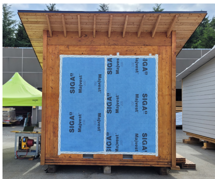
Figure 3. RAIN chamber with the mock-up wall installed (source: FPInnovations).
