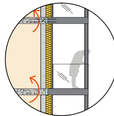
**Exterior supported balconies** (or self-supporting balconies) are supported from below. This allows the size of the tie-backs that connect the balcony to the building to be minimized, reducing thermal bridging.
