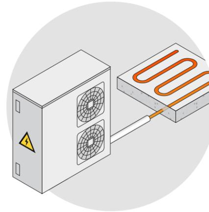
\* "Hydronic" refers to the practice of using a water-based medium to distribute heat throughout a building. Hydronic systems can use either radiators, in-floor systems, and in some cases, in-ceiling systems.
