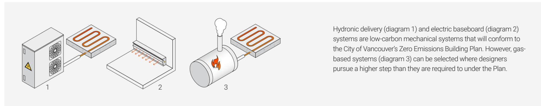
Hydronic delivery (diagram 1) and electric baseboard (diagram 2) systems are low-carbon mechanical systems that will conform to the City of Vancouver's Zero Emissions Building Plan. However, gas-based systems (diagram 3) can be selected where designers pursue a higher step than they are required to under the Plan.
