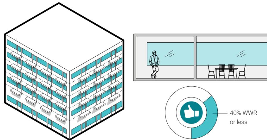
Reducing the size of windows can actually help to improve occupants’ comfort by reducing glare and providing a more comfortable indoor temperature, without requiring any additional indoor lighting or losing the potential for views.
