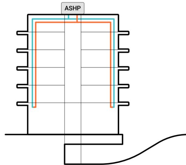
Cooling provided by heat pumps can be distributed by either a centralized or decentralized system.
