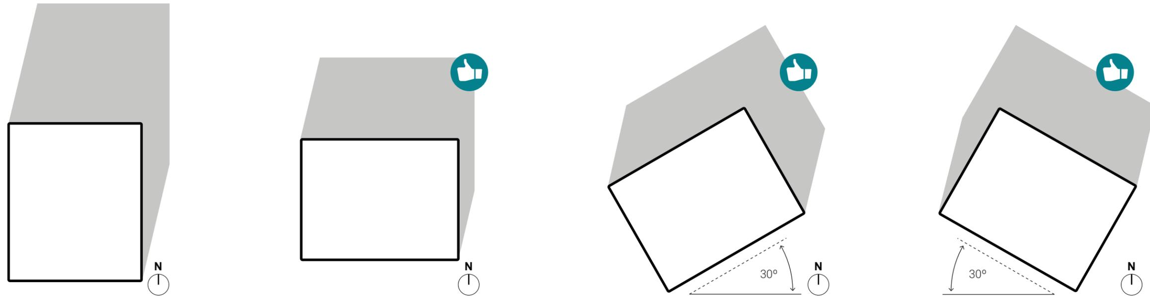
Professionals who orient their buildings to maximize solar-gain potential from the south can reduce heating demands by as much as 30 to 40%. While this strategy does not minimize heat losses per se, it does take advantage of passive heat gains that can provide a benefit when reaching for a TEDI target.
