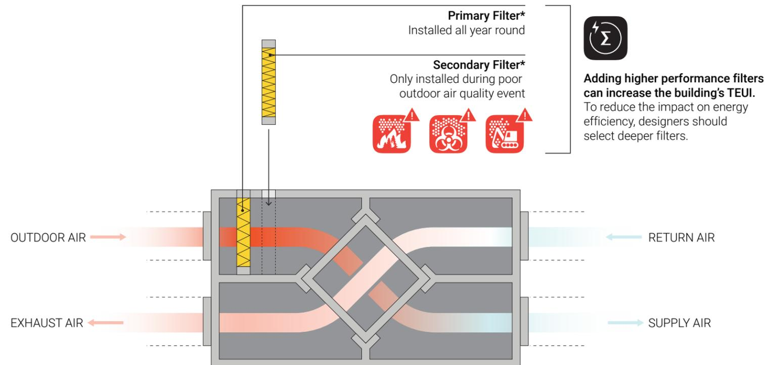
\*Note that filters can be either internal to the unit, or external downstream of the supply fan.
