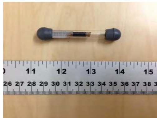
Figure 7.2 Typical CATS used for PFT testing at the case study building
