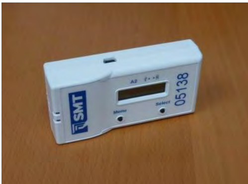
Figure 3.3 SMT-A2 unit. An LCD screen is provided to interact with the unit. Temperature and relative humidity sensors are located within the unit, and ports are provided on the bottom of the unit to attach external sensors.
