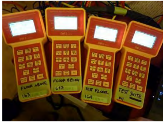
Figure 5.7 Four Retrotec DM-2 gauges used for control of the fans and pressure measurements during the testing. The gauge for the test zone is connected to a laptop running Retrotec's FanTestic airtightness testing software to record data points.
