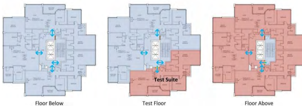
Figure 5.5 Airtightness testing layout for pressurization of an -01 suite while equalizing the floor above showing the direction or airflow between zones either through open doors to allow for free movement of air, or as forced into zones by the testing fans.
