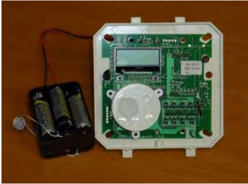
Figure 3.1 SMT-A3 unit with attached battery pack shown without faceplate. An LCD screen is provided to interact with the unit. Temperature and relative humidity sensors are located to the left of the LCD screen; the CO 2 sensor is round and white, and the pressure sensor is located on the back of the unit with a tube running out to a hole on the middle top of the right side.
