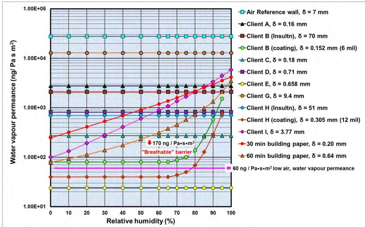
Figure 3 – Water vapour permeance of sheathing membranes as a function of RH used in respective Client drainage systems;  $\delta$  = thickness of membrane or insulation product
