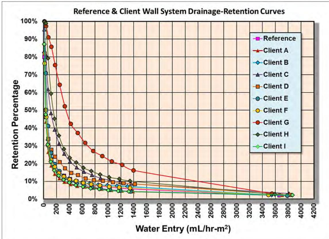
**Figure 4 – Reference and Client wall system Drainage-Retention Curves**
