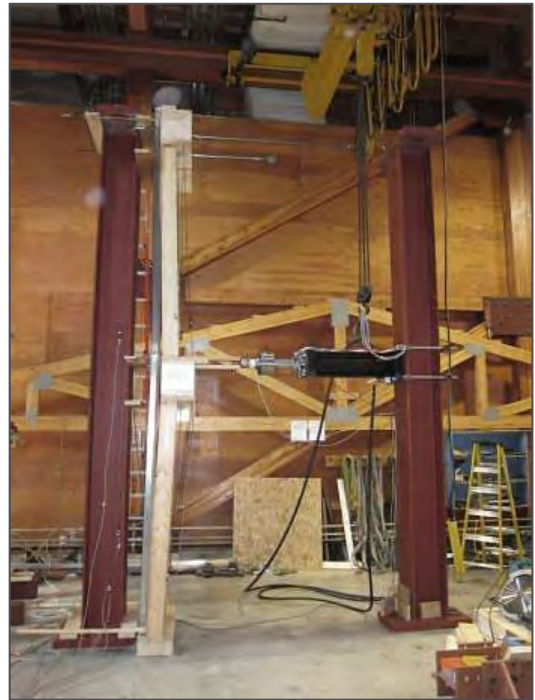
b) deformation of wall framing under load
