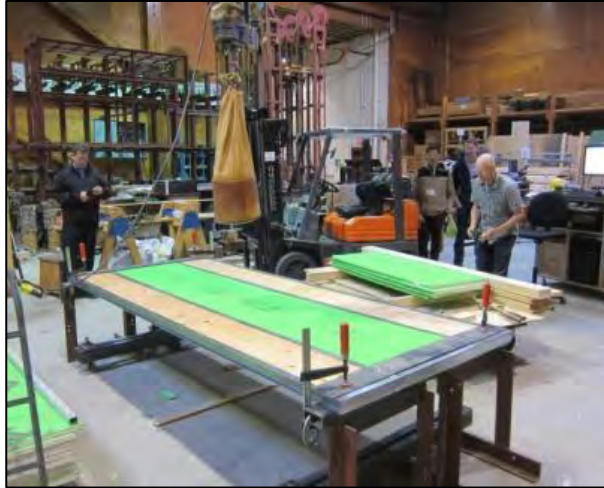
a) 1/2" plywood on each side
