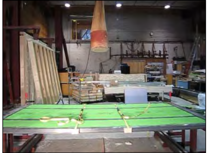
b) small wood blocks and straps tied at outer edges of H-studs
