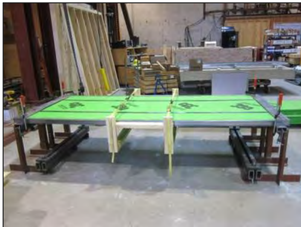
c) wooded frame and straps tied at outer edges of H-studs
