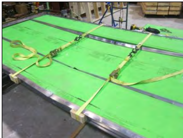
Figure 13 Center H-studs buckling/rotating
