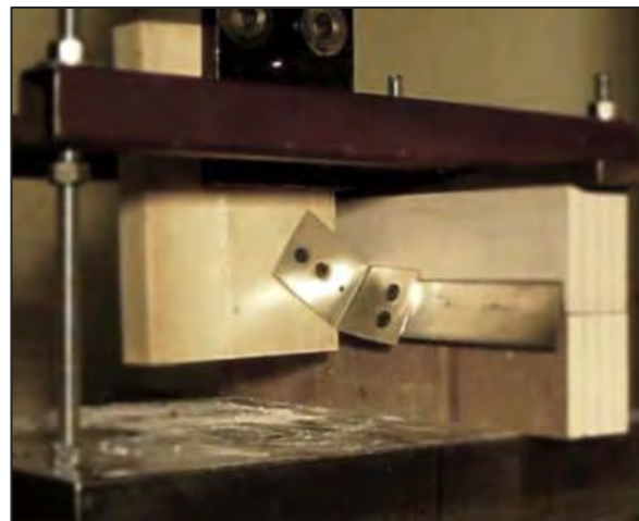
Figure 26 Twist of aluminum clips under load condition C
