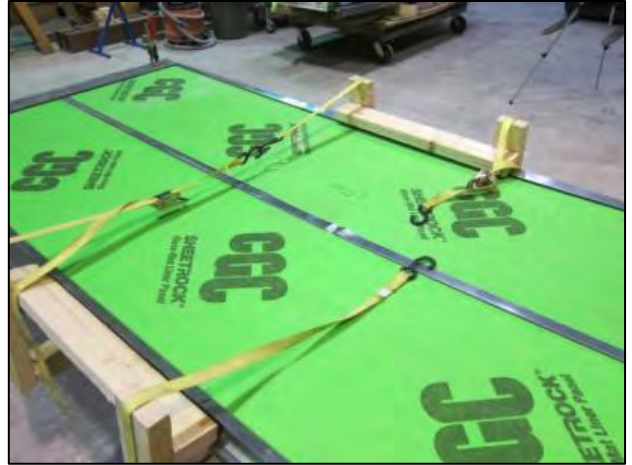
Figure 16 Center H-stud damage for 2 panels
