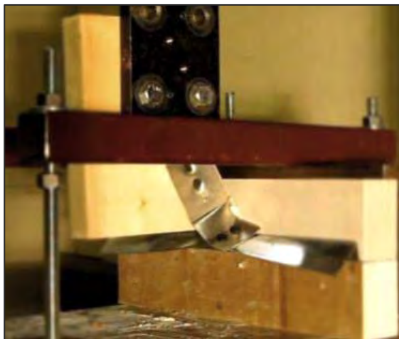
c) Failure of clips under load condition C
