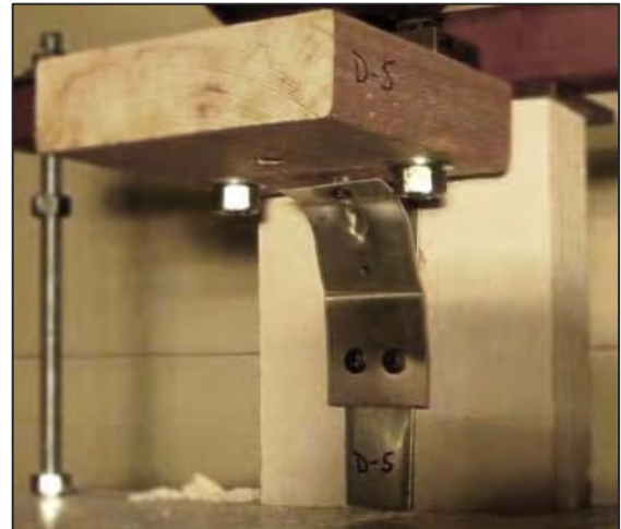
b) Failure of clips under load condition B
