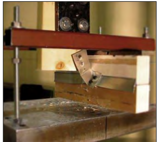
d) Failure of clips under load condition C
