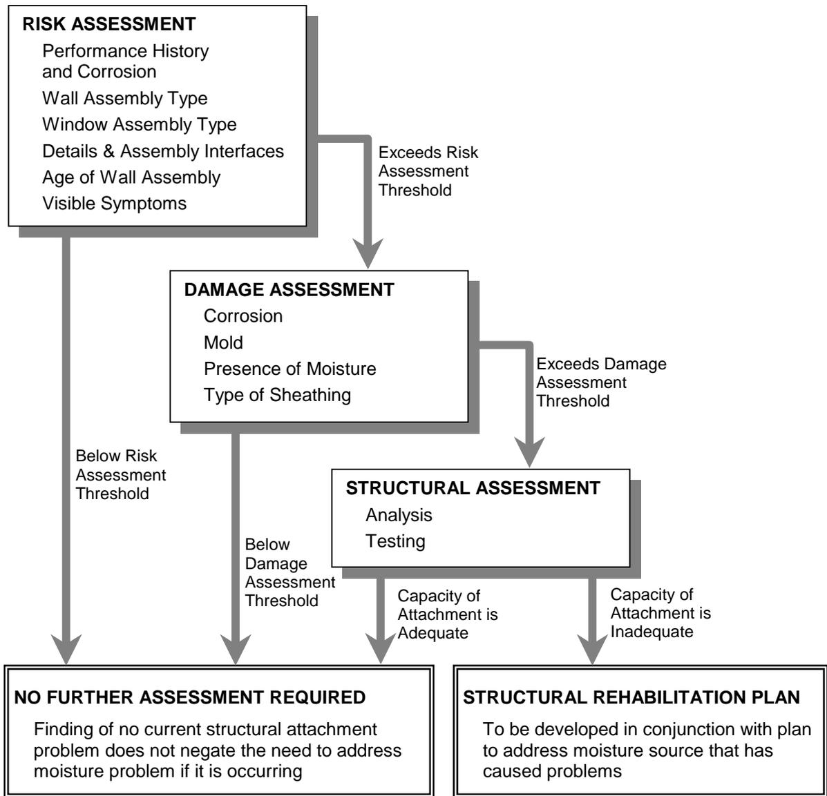
**Figure A-1: Assessment of Structural Attachment of Cladding Process**
