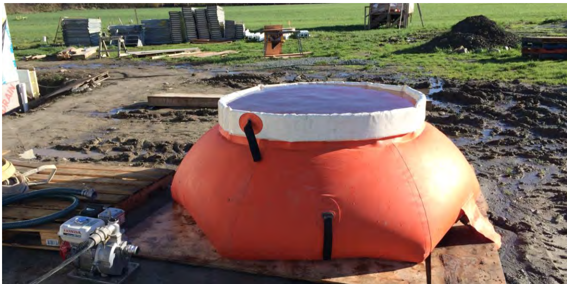
Fig. 3.2.5 Water bladder and pump used to deliver water at consistent pressure to the calibrated rain rack.
