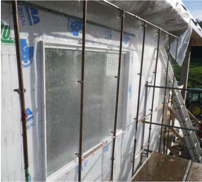
Fig. 3.2.3 Calibrated rain rack installed to spray sample with water. Rain rack was oversized to spray window and surrounding ICF wall area.
