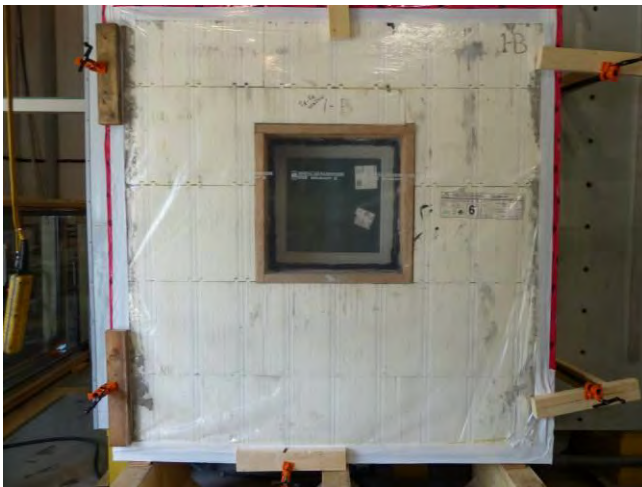
Fig. 3.1.1 Air Leakage Testing
