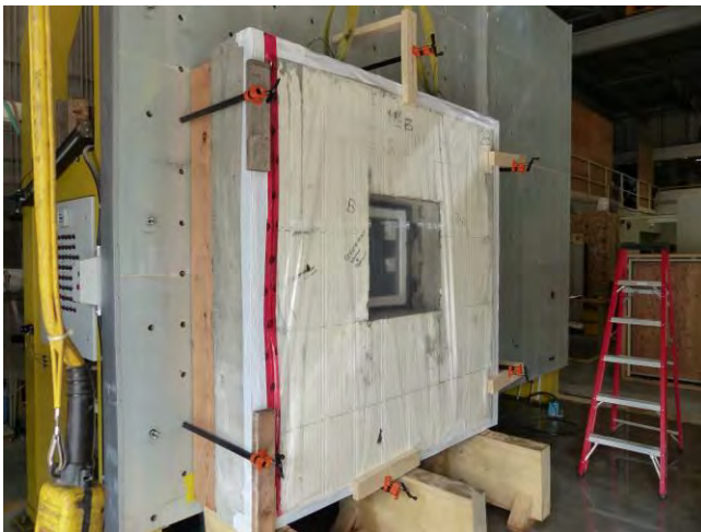
Fig. 3.1.2 Air Leakage Testing
