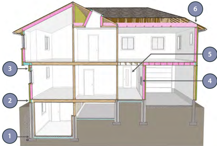
Figure 2: Typical Problem Areas for Insulation Continuity
