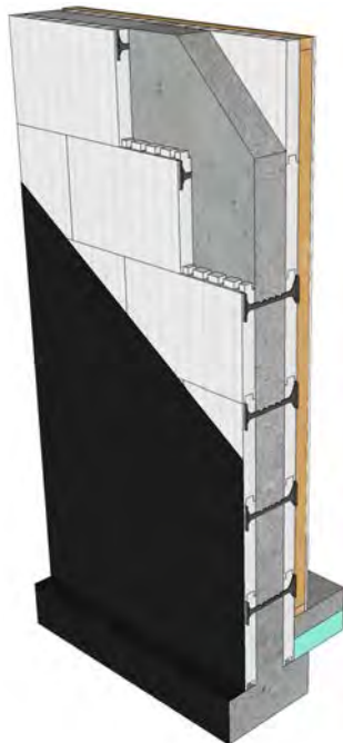
Basement Wall Insulated with ICF
