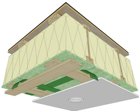
*Sealed Interior Sheathing Approach (with Service Cavity)*
