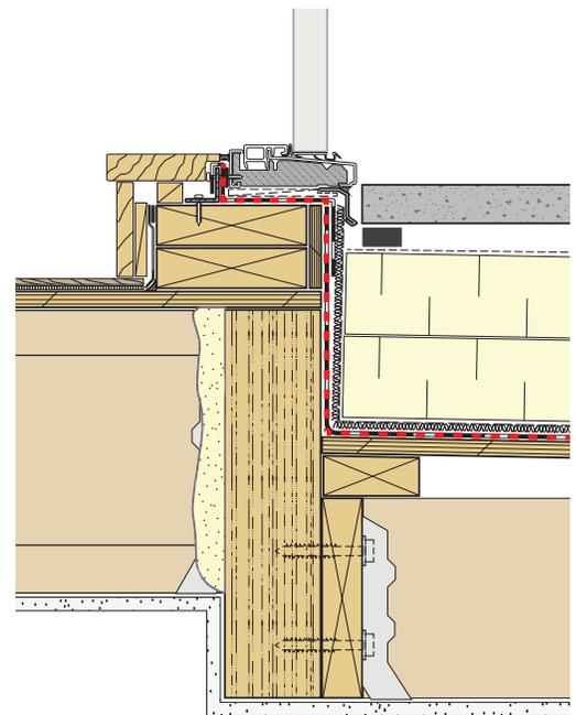
*Inverted roof deck with dropped framing and continuous waterproof roof membrane from door sill to curb/field membrane (red dash)*
