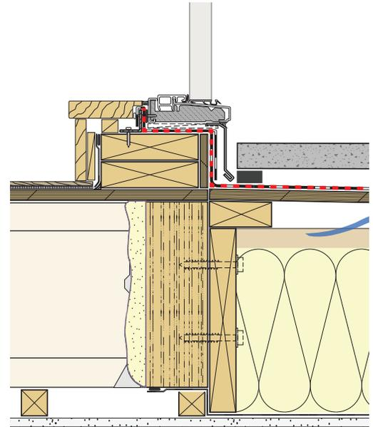
*Vented roof deck with dropped framing and continuous waterproof roof membrane from door sill to curb/field membrane (red dash)*
