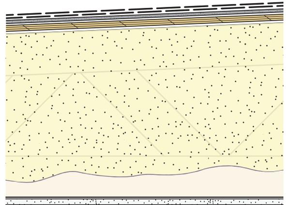
*Joist-Insulated Unvented Flat Roof*
