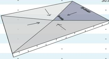
**Sloped insulation effective R-value calculations from the supplier** | Some roofing material suppliers offer assistance in designing the sloped roof insulation (also referred to as the taper package), including the calculation of its effective R-value. However, they should confirm that the calculation uses the integrated area-weighted approach rather than the simple average insulation thickness.
