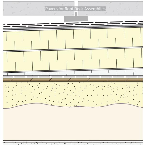
Split-Insulated Exposed Membrane Flat Roof
