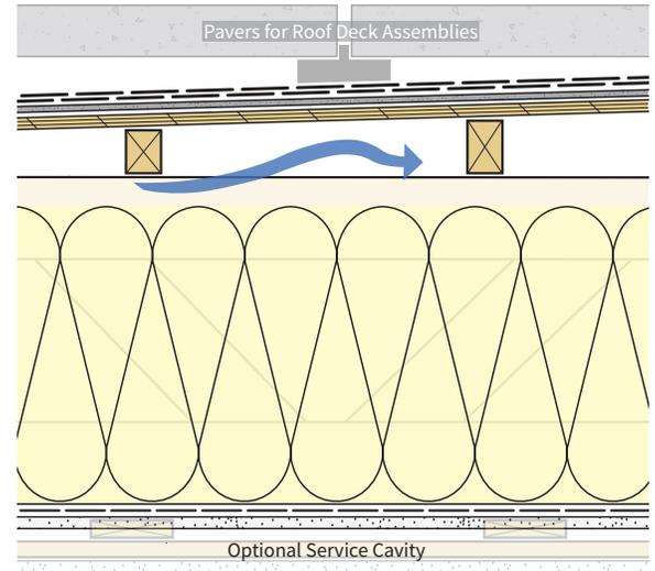
Joist-Insulated Vented Flat Roof
