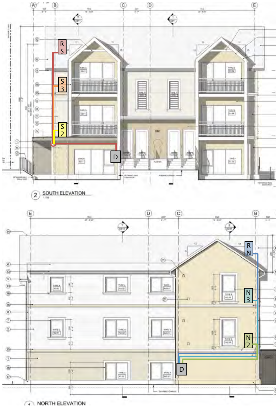
Figure 3-4- North and South elevations showing approximate locations for the instrumented enclosure sections. 6
