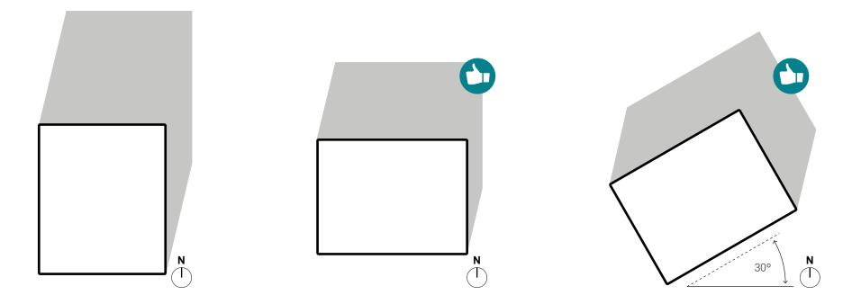
Professionals who orient their buildings to maximize solar-gain potential from the south can reduce heating demands by as much as 30 to 40%. While this strategy does not minimize heat losses per se, it does take advantage of passive heat gains that can provide a benefit when reaching for a TEDI target.
