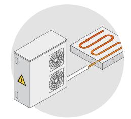
\* "Hydronic" refers to the practice of using a water-based medium to distribute heat throughout a building. Hydronic systems can use either radiators, in-floor systems, and in some cases, in-ceiling systems.
