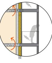
Exterior supported balconies (or selfsupporting balconies) are supported from below. This allows the size of the tie-backs that connect the balcony to the building to be minimized, reducing thermal bridging.
