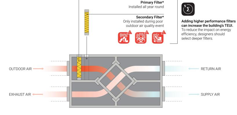
\*Note that filters can be either internal to the unit, or external downstream of the supply fan.
