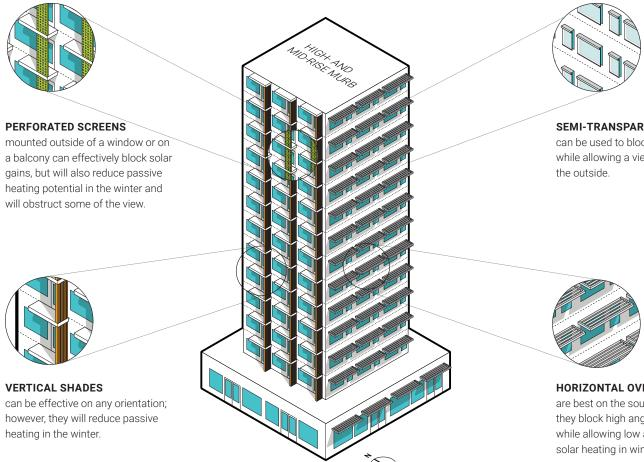
SEMI-TRANSPARENT SHADES can be used to block solar gains while allowing a view through to
