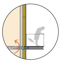
Thermally-broken balconies use lower-conductivity materials (such as stainless steel) to attach the balcony to the building, reducing heat losses through the envelope.
