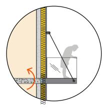
Exterior hung balconies (or suspended balconies) are attached to the building by tension cables. These allows for continuous insulation across the building envelope.
