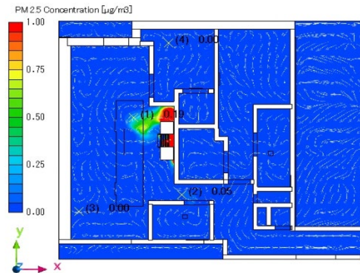
Figure 180. Plan 1 with contaminant concentration and velocity vector.
