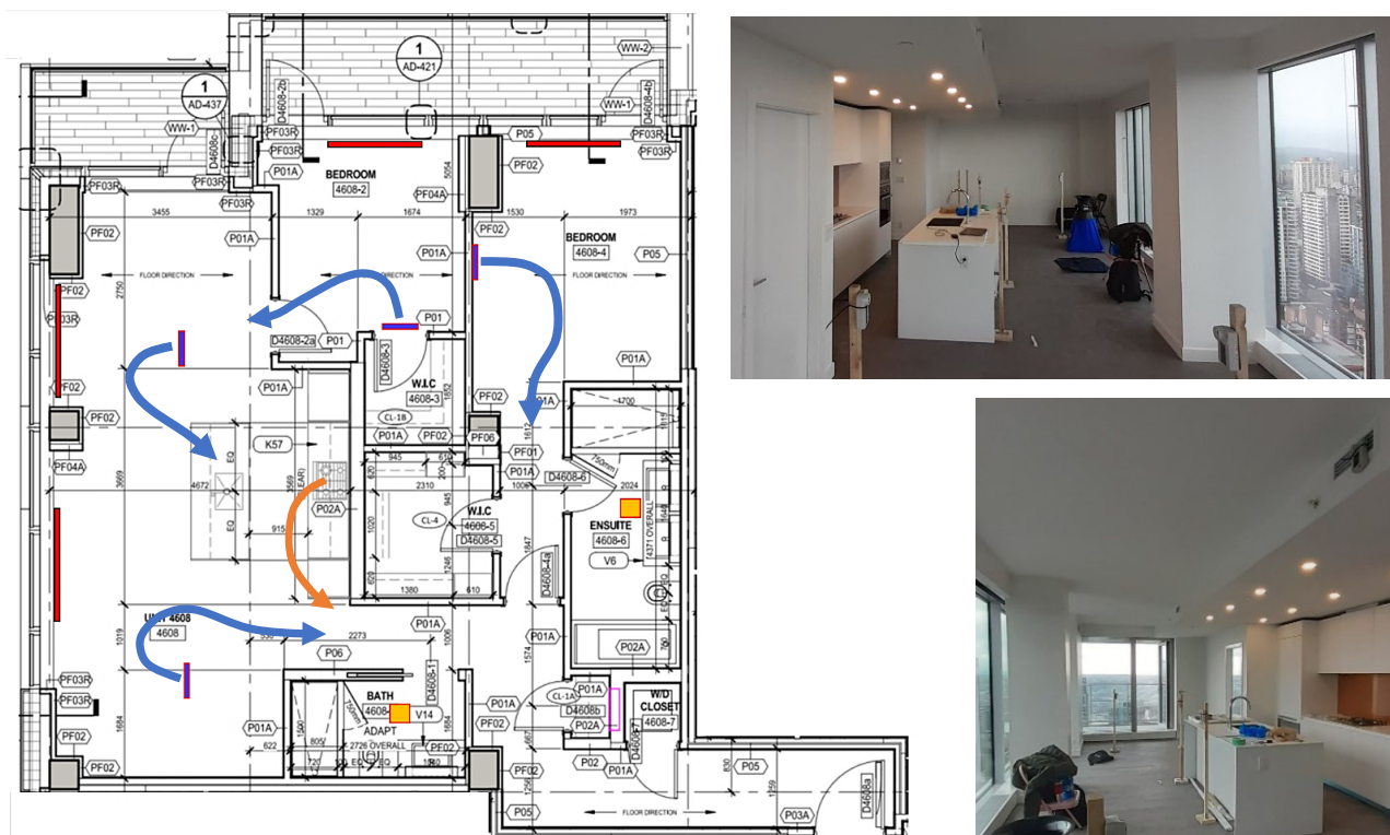
Figure 104. Left. Suite C: baseboard heaters shown in red, anticipated cascading ventilation shown with blue arrows, return diffusers shown in yellow, kitchen pollutant shown with yellow arrow. Right. CO 2 monitoring loggers placed in the rooms
