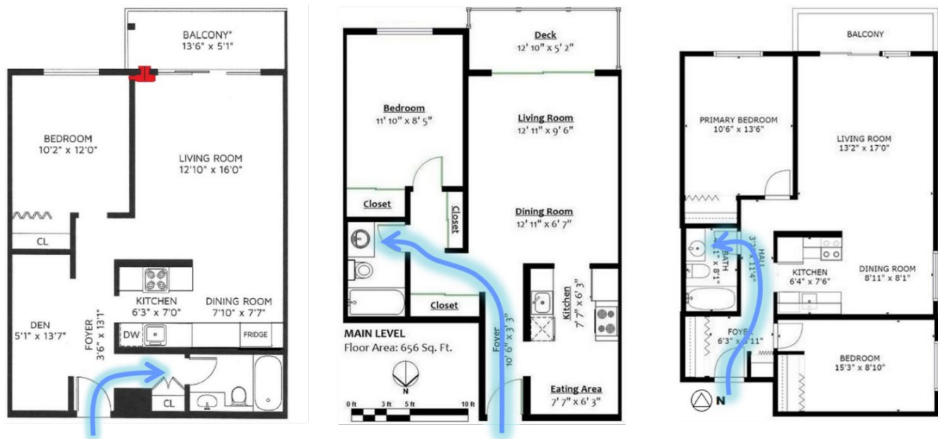
Figure 80. Corridor pressurization ventilation air bypasses the main rooms in a suite (exhaust fan in bathroom)
