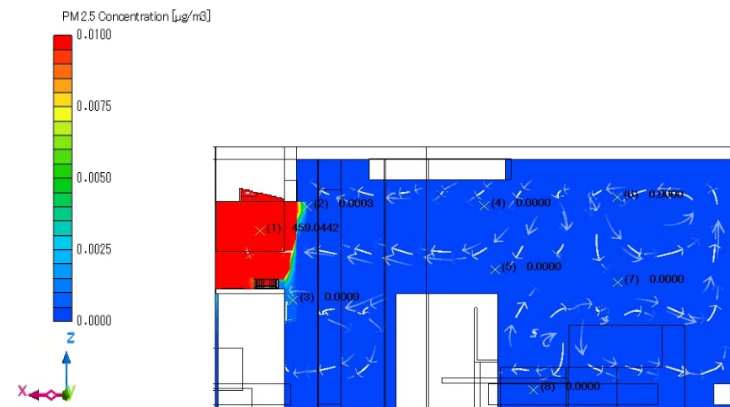
Figure 188. Section 1 with contaminant concentration and velocity vector.
