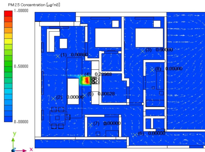
Figure 184. Plan 1 with contaminant concentration and velocity vector.
