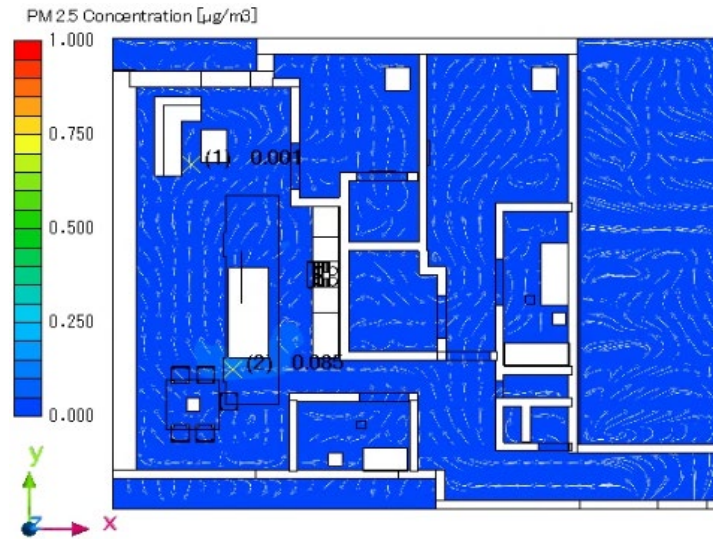
Figure 180. Plan 1 with contaminant concentration and velocity vector.
