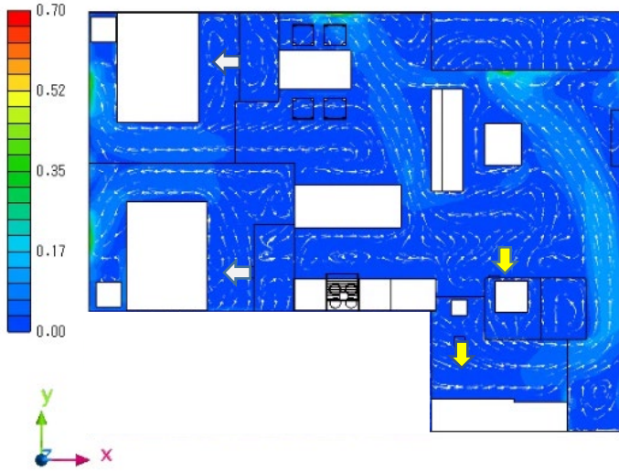
Figure 147. Plan 1, z = 0.2 m, magnitude of velocity and velocity vector.
